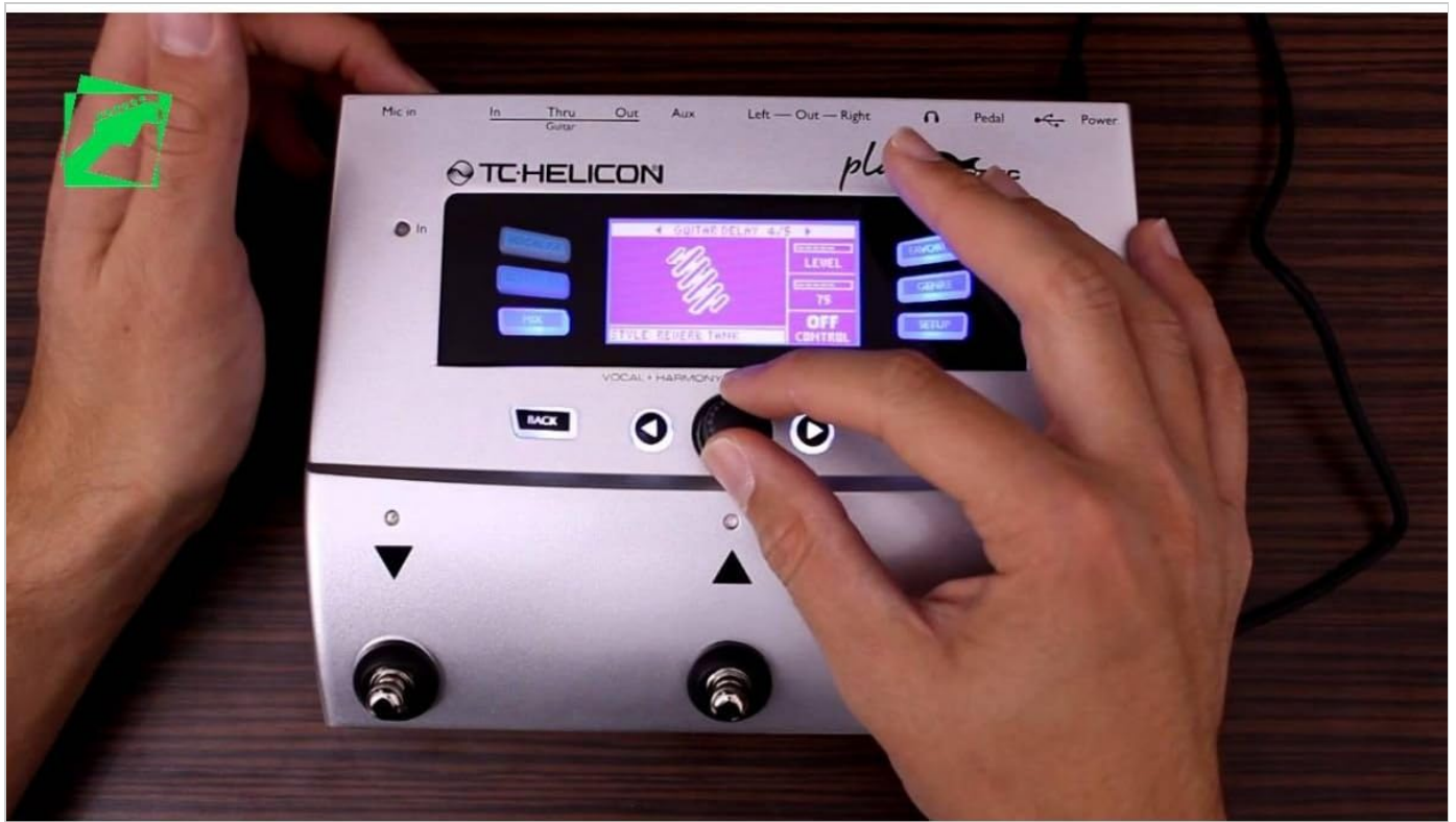
Figure 3.2.1: Close-up of the TC Helicon Play Electric's user interface, showing the display, navigation buttons, and rotary encoder.
