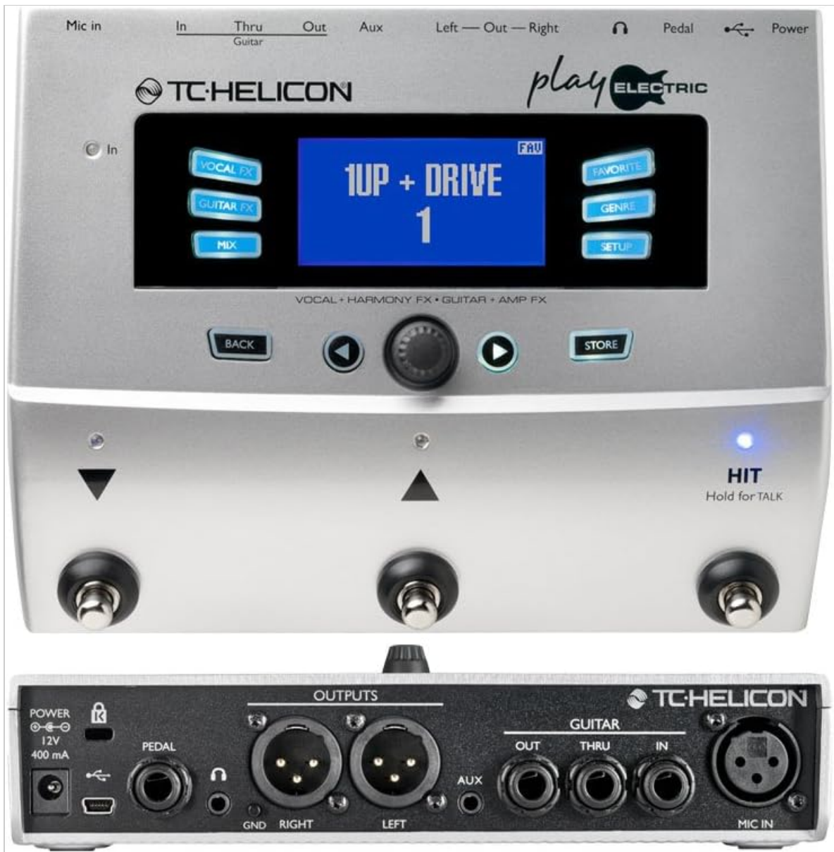
Figure 2.2.1: Front panel overview of the TC Helicon Play Electric, showing microphone input, guitar input/output, and main display.
