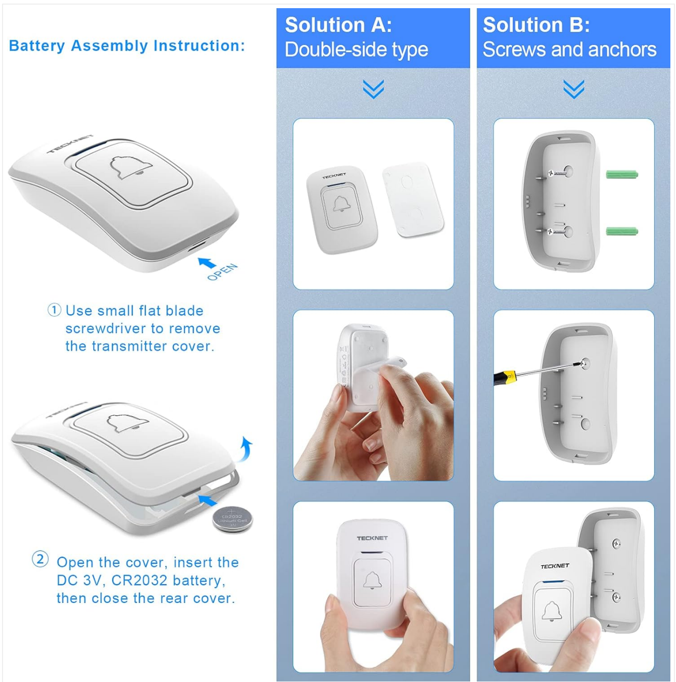
Figure 4.1: Step-by-step guide for installing the CR2032 battery in the doorbell transmitter by opening the back cover.
