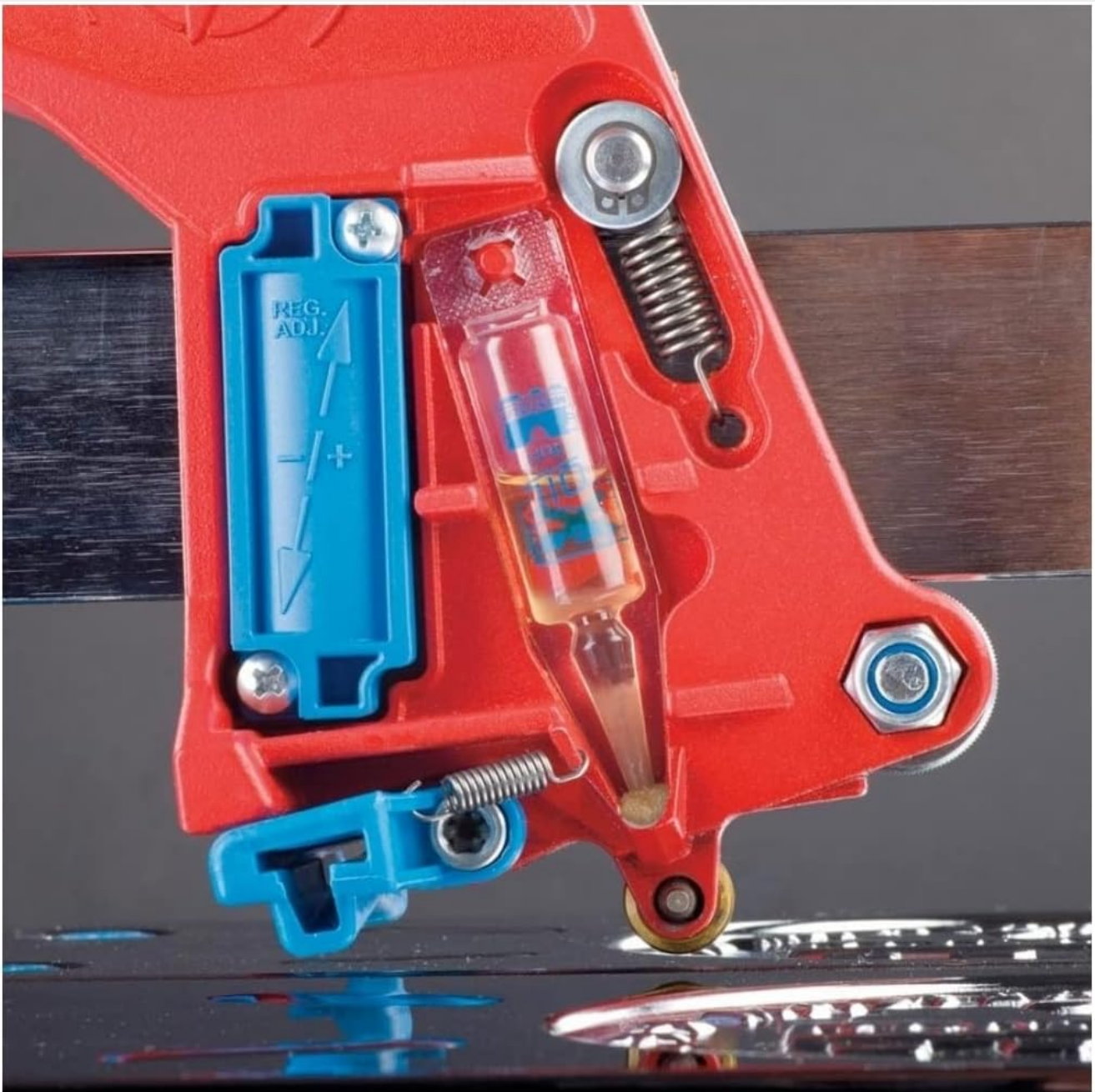
Figure 5.1: Detail of the scoring wheel assembly, showing the fluid reservoir for enhanced scoring.
