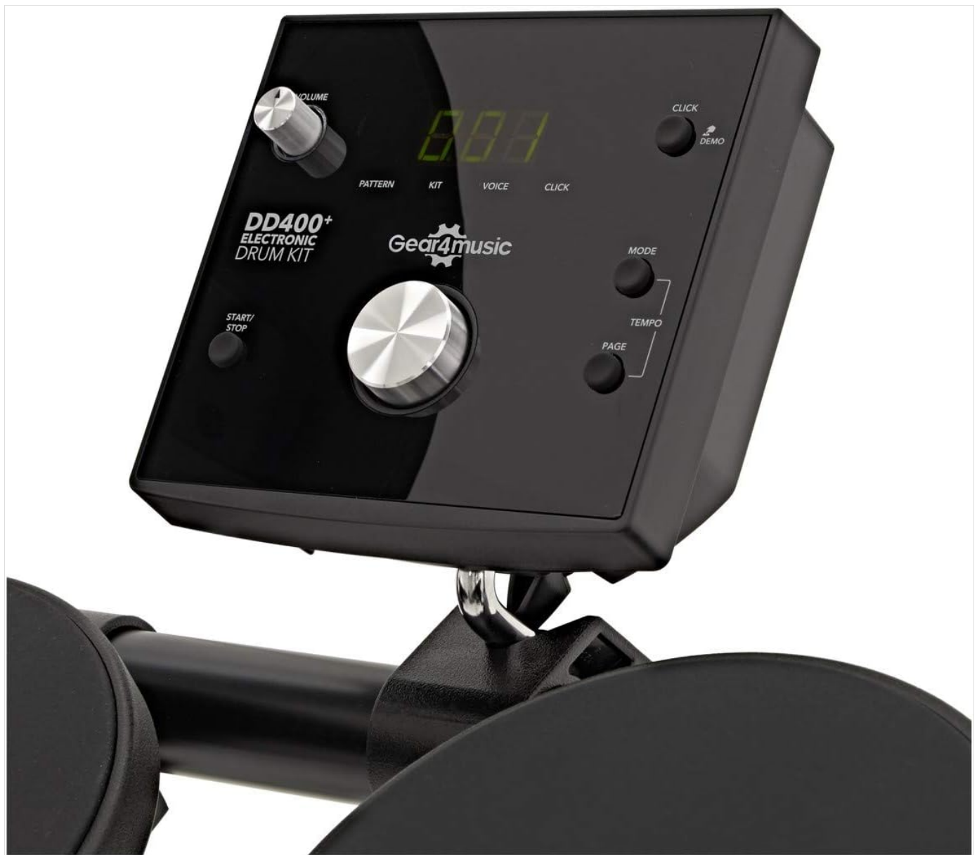
Figure 4.3: Detailed view of the DD400 control module. It features a volume knob, pattern, kit, voice, click, demo buttons, mode, tempo, page buttons, and a start/stop button, along with a digital display.
