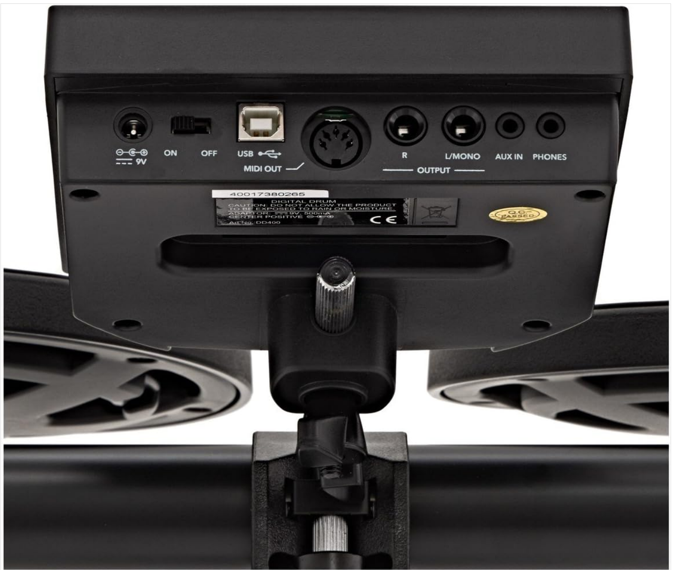
Figure 4.4: The rear panel of the DD400 module showing various input/output ports. These include a 9V DC power input, ON/OFF switch, USB port, MIDI OUT, R/L MONO OUTPUT, AUX IN, and PHONES output.
