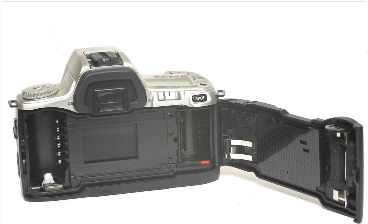
Figure 4: Rear view of the camera with the film door open, revealing the film chamber on the left and the film take-up spool on the right, ready for film loading.
