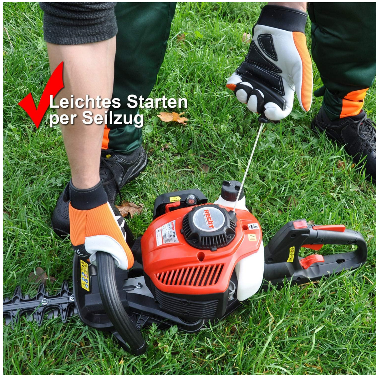
Figure 4: Demonstrating the pull cord starting procedure.
