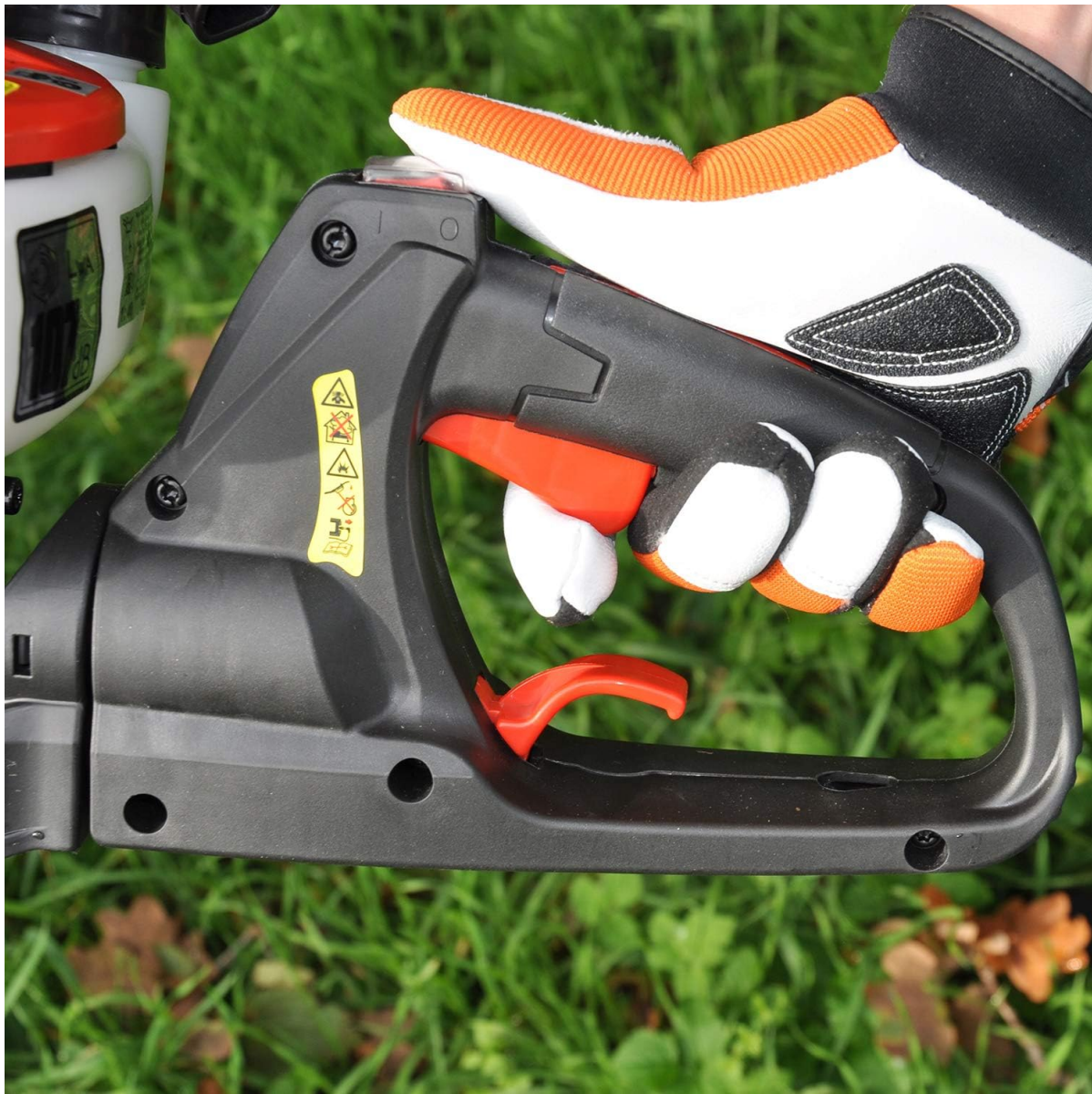
Figure 6: Proper hand placement on the handle and trigger during operation.
