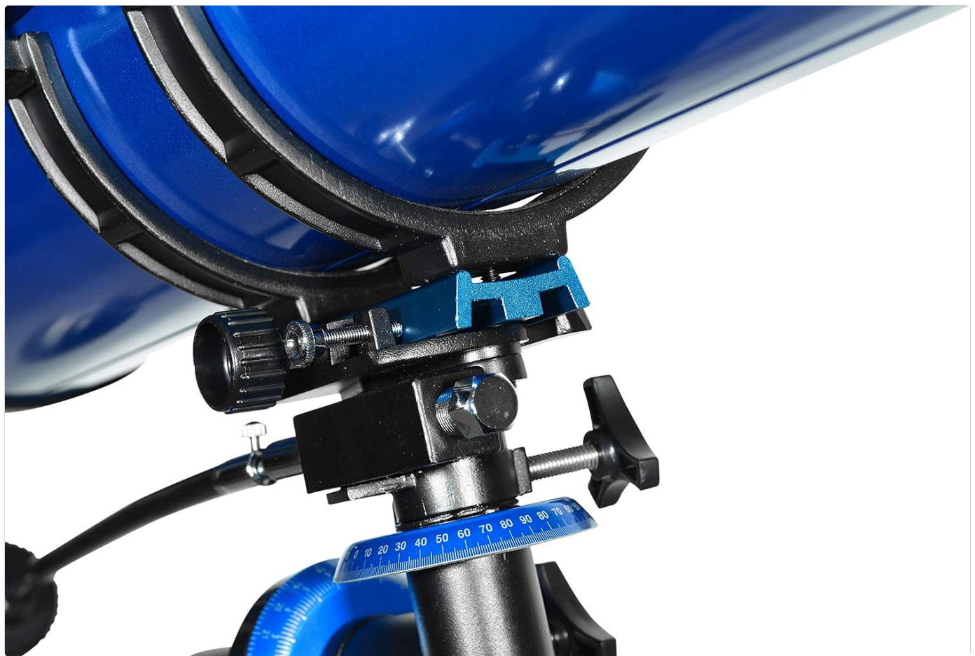
Figure 3: German Equatorial Mount with slow motion controls.
