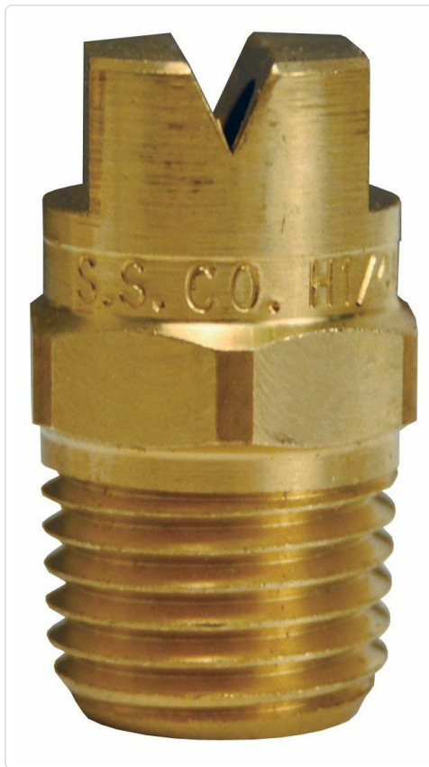
Figure 1: Dixon NZ4040S High Pressure Spray Soap Nozzle. This image displays the Dixon NZ4040S high-pressure spray soap nozzle. It is a brass-colored, cylindrical component with a threaded male inlet at the bottom for attachment. The top features a V-shaped opening designed to produce a 40-degree fan spray pattern, suitable for soap application. The body of the nozzle has hexagonal sections for wrench grip and engraved text, including 'S.S. CO.' and 'HI'.
