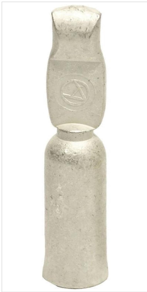
Figure 1: Anderson Power Products 5915-BK PowerPole Contact. This image shows a single copper contact, designed for crimping onto 10 or 12 AWG wire. The contact features a flat, spade-like end for insertion into a PowerPole housing and a cylindrical barrel for wire crimping.
