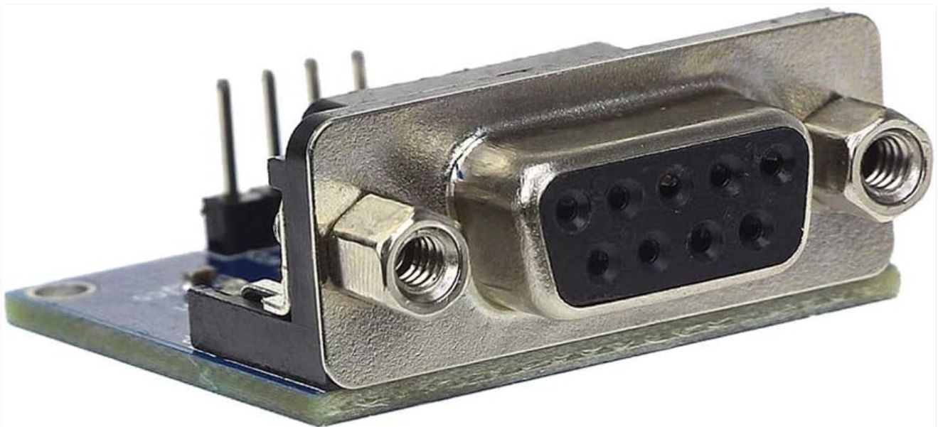
Figure 3: This image shows the standard 9-pin D-sub (DB9) male connector, which provides the RS232 interface for the module.
