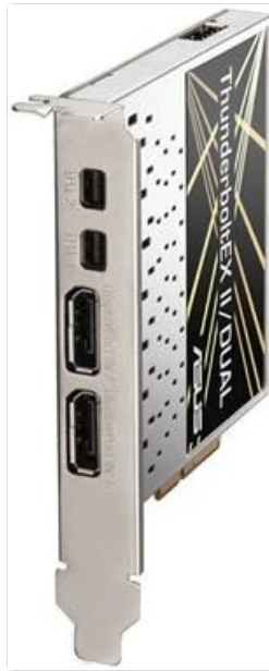
Figure 2: Side view of the ASUS ThunderboltEX II/DUAL Adapter card, highlighting the two Thunderbolt 2 ports and the DisplayPort input.
