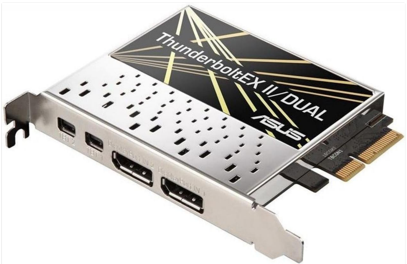
Figure 1: Top-down view of the ASUS ThunderboltEX II/DUAL Adapter card, showing the PCIe connector and the two Thunderbolt 2 ports.
