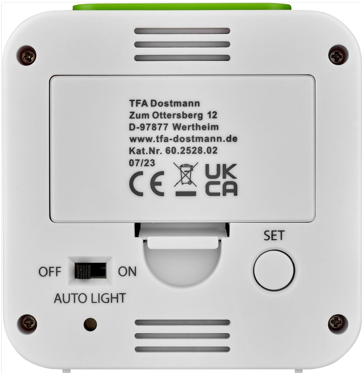
Figure 2: Rear view with battery compartment and controls.
