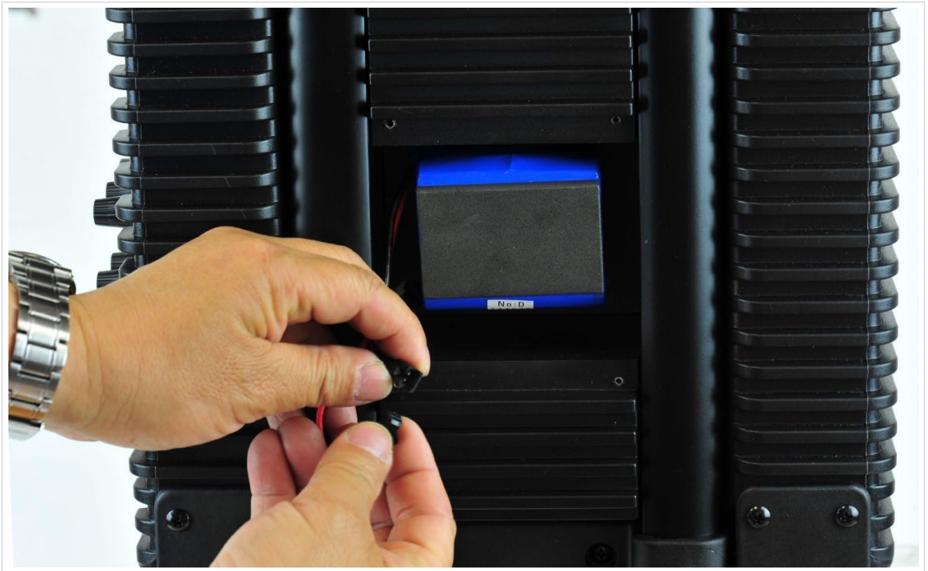
Figure 5.1: Illustrates the process of connecting the internal rechargeable battery within the HS700 unit.
