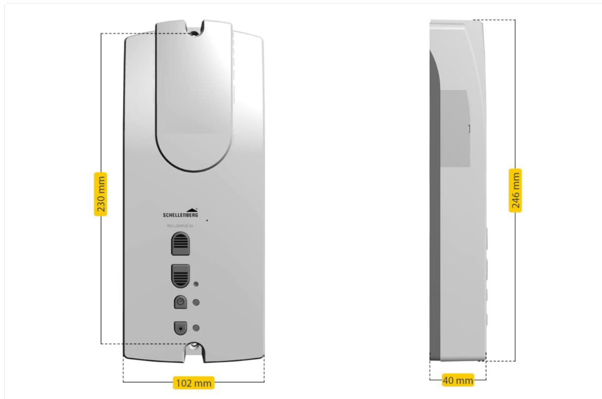
Figure 9.1: Dimensions of the Rolldrive 55 unit.
