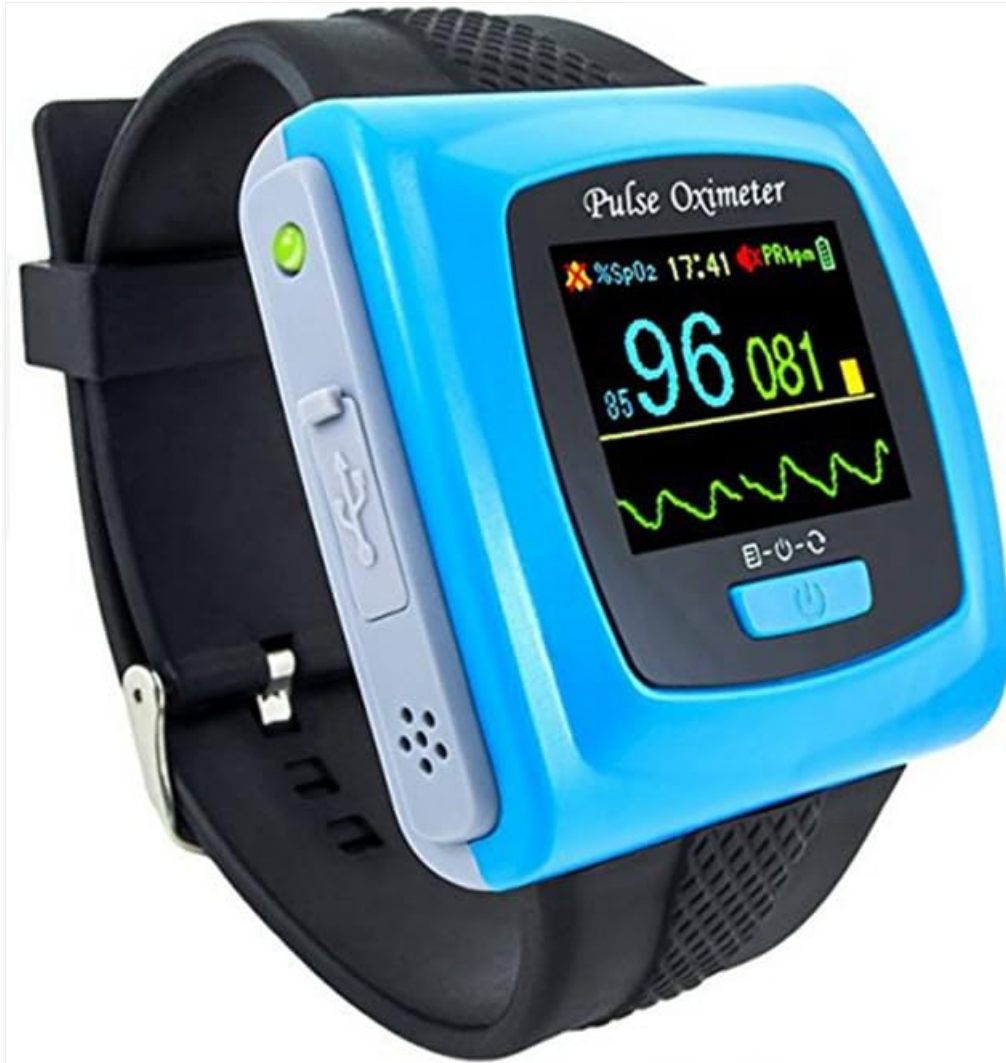
Figure 2: Side view of the CMS50F unit, showing the USB port for charging and data transfer.
