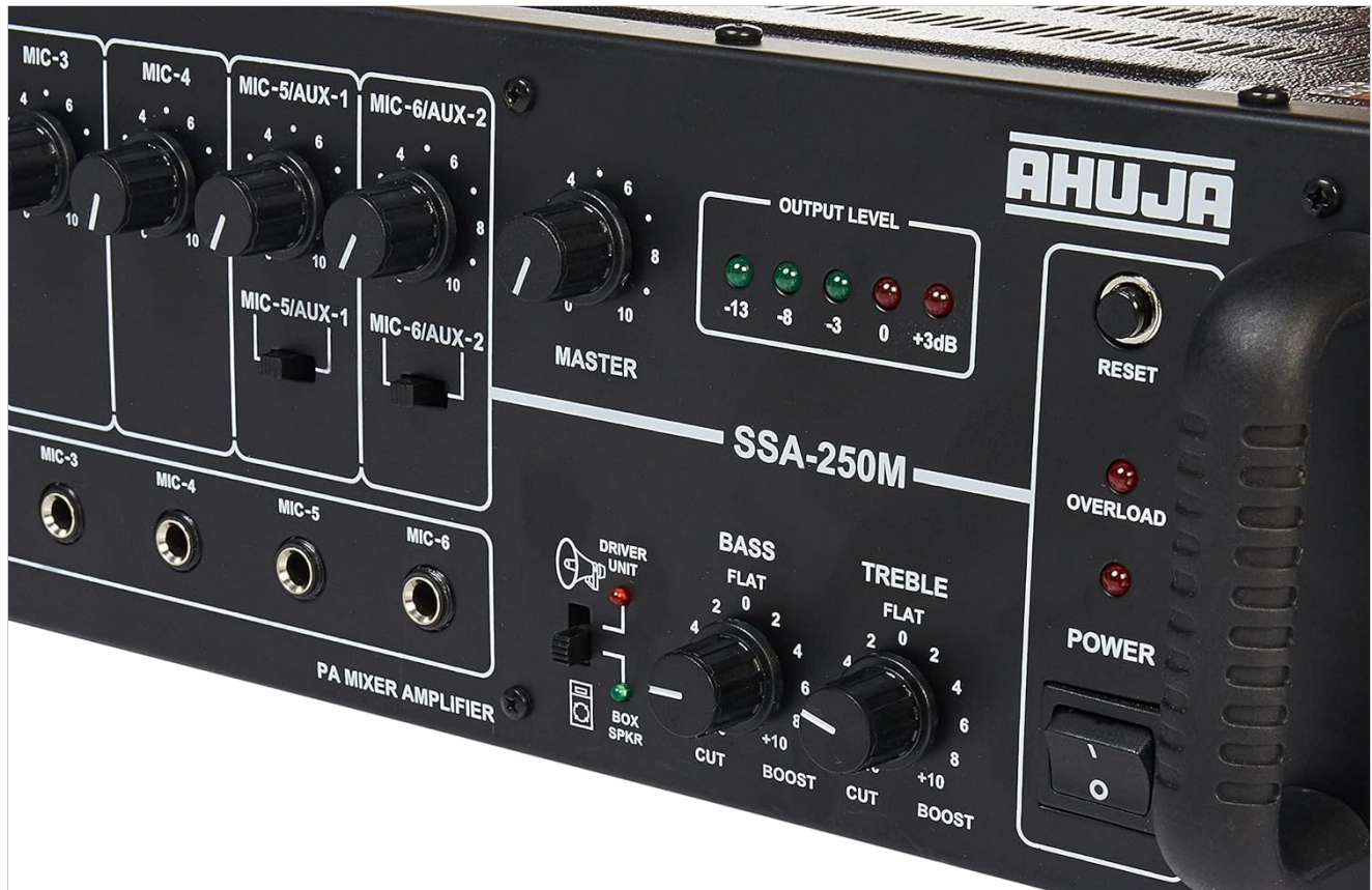
Image: Close-up view of the Ahuja SSA250M amplifier's front panel, showing individual microphone and auxiliary input level controls, master volume, bass and treble tone controls, output level indicators, and power/overload indicators.
