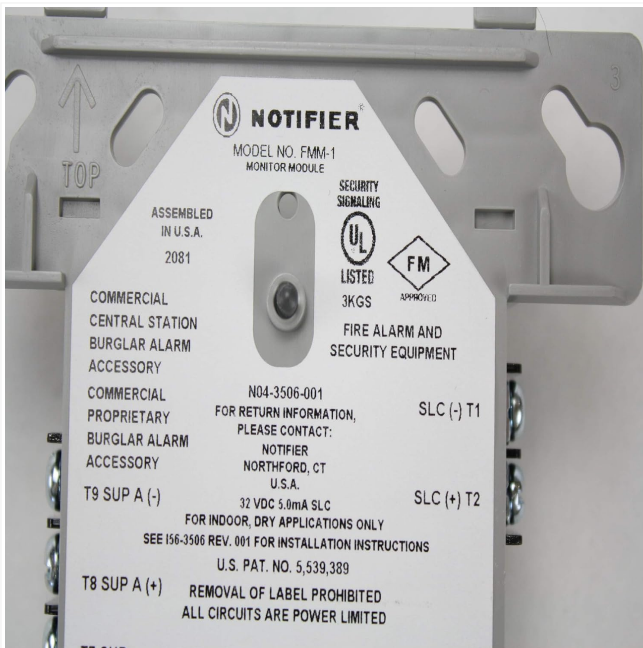
Figure 3: Rear view of the Notifier FMM-1 module with wiring details. This image provides a clear view of the terminal block for connecting to the fire alarm system's Signaling Line Circuit (SLC) and the initiating device circuit (IDC), along with product labels and certifications.
