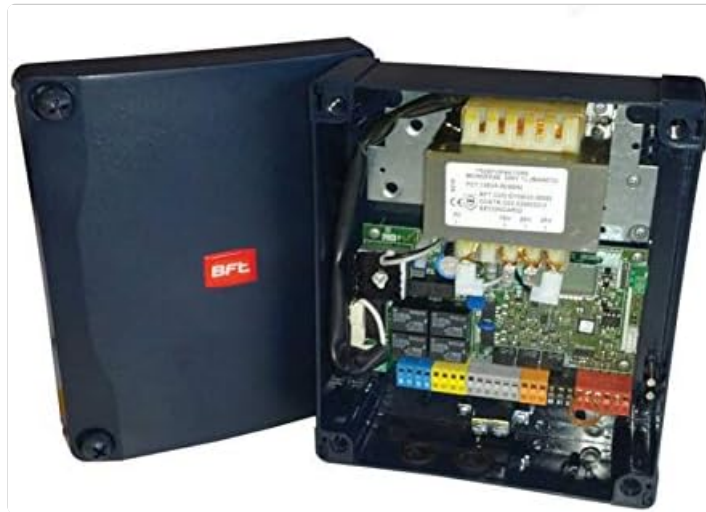
Figure 1: The BFT THALIA control unit with its protective cover open, revealing the internal circuit board, transformer, and various terminal blocks for electrical connections. The BFT logo is visible on the closed part of the casing.
