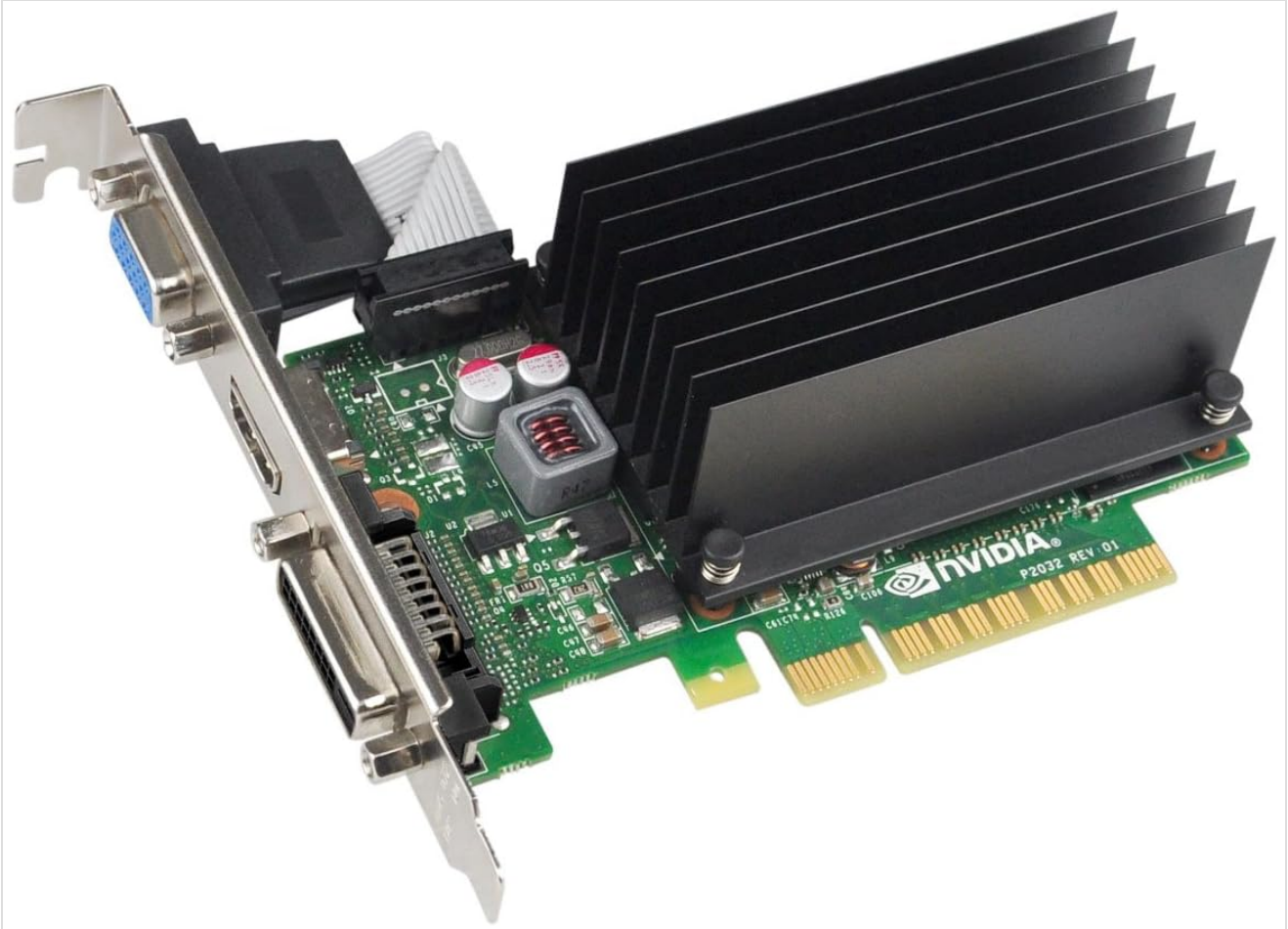
Image 3.1: Angled view of the EVGA GeForce GT 730, showing its compact design.
