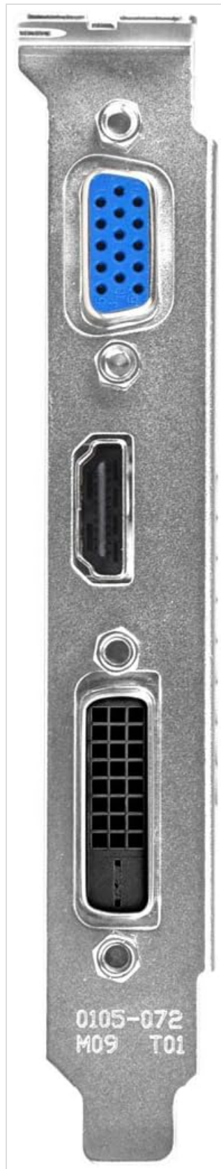
Image 4.1: Rear view of the graphics card displaying the DVI, HDMI, and VGA output ports.
