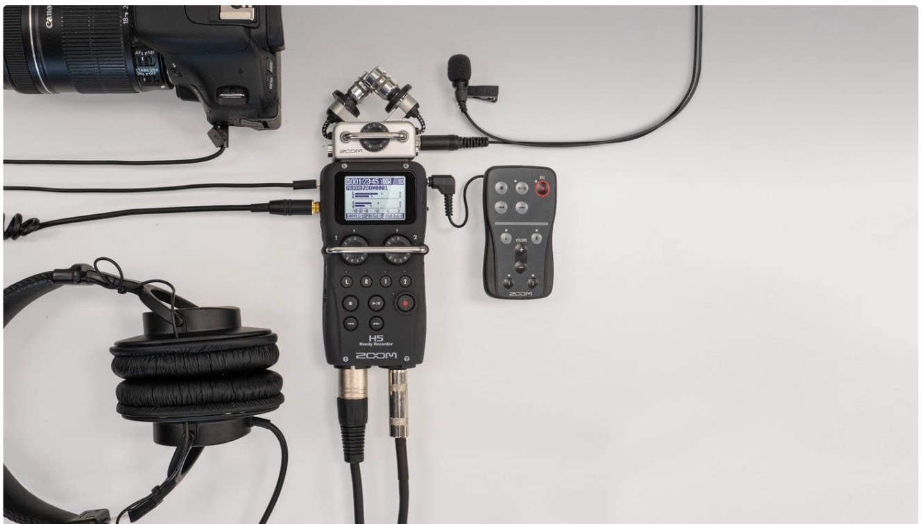
Figure 3: The Zoom H5 Handy Recorder displayed with some of its common accessories, including headphones, a remote control, and various cables, illustrating a typical recording setup.
