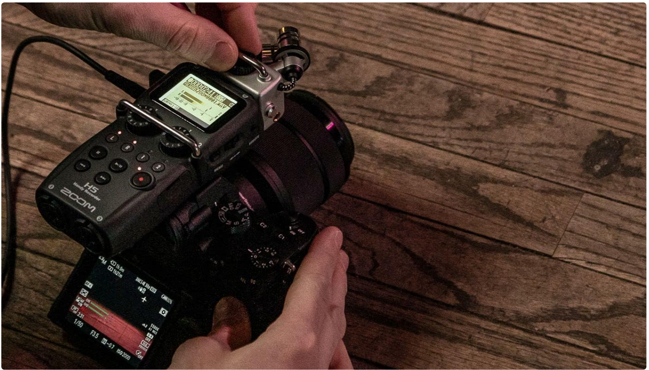
Figure 4: The Zoom H5 Handy Recorder mounted on top of a camera, demonstrating its use as an external audio recorder for video production, enhancing sound quality.
