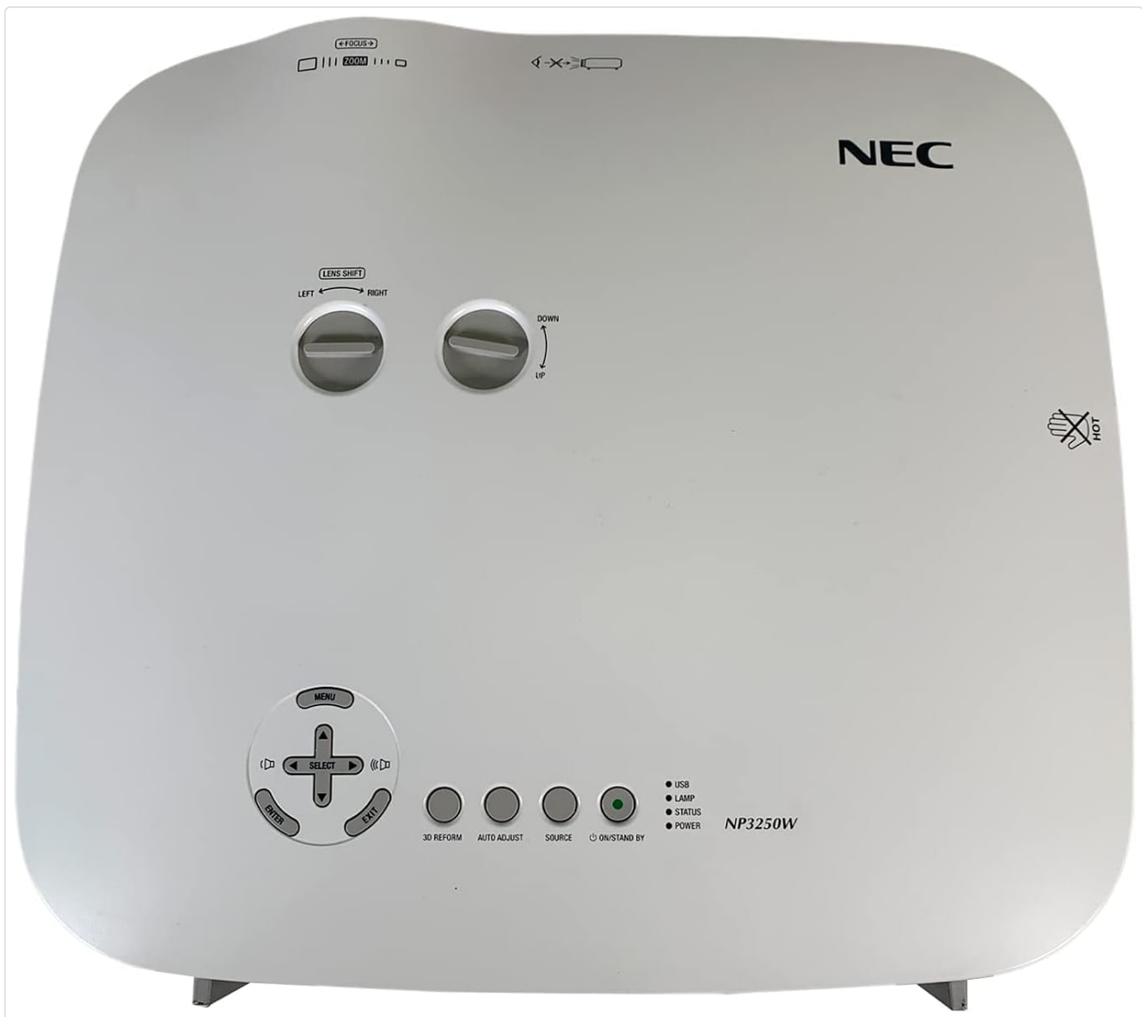
Figure 3.3: Top panel controls of the NEC NP3250W projector, including navigation buttons (Menu, Select, Enter, Source, Auto Adjust, 3D Reform), indicator lights (USB, Lamp, Status, Power), and lens shift/focus adjustment dials.
