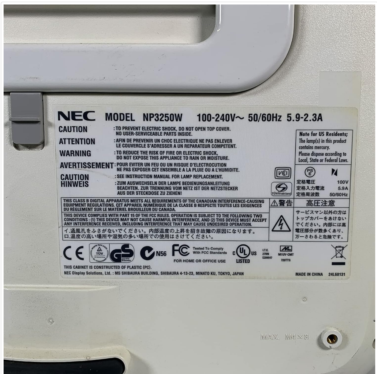
Figure 3.6: Bottom label of the NEC NP3250W projector, displaying model number (NP3250W), electrical ratings (100-240V~
