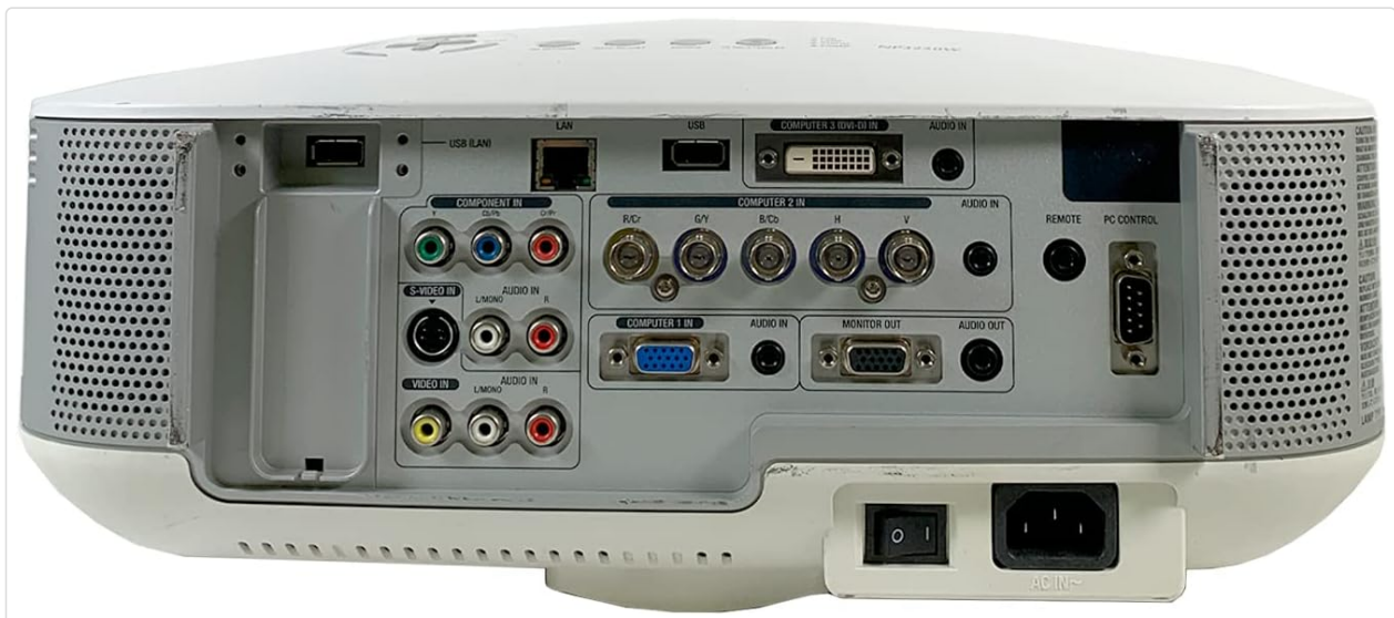
Figure 3.4: Rear panel of the NEC NP3250W projector, detailing all input/output ports including USB (B/LAN), LAN, USB, Computer 1/2 (VGA/DVI-D), Component In, S-Video In, Video In, Audio In/Out, Remote, PC Control, and AC In power connection.
