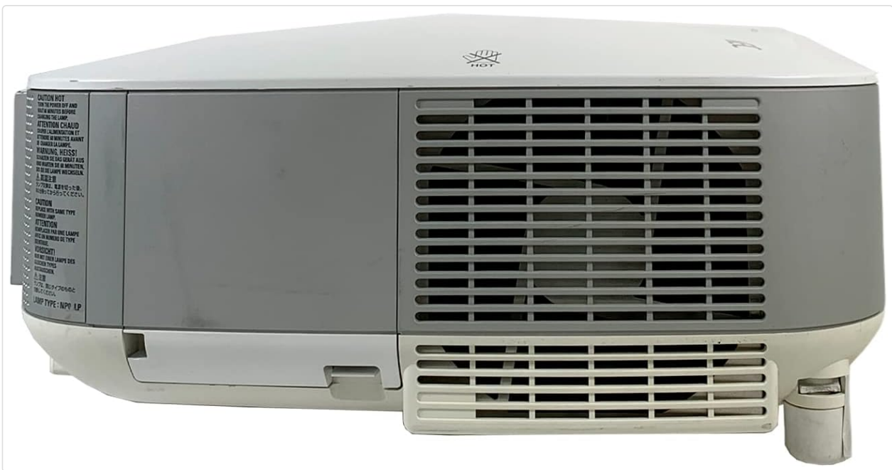
Figure 3.5: Side view of the NEC NP3250W projector, emphasizing the large ventilation grilles for heat dissipation.
