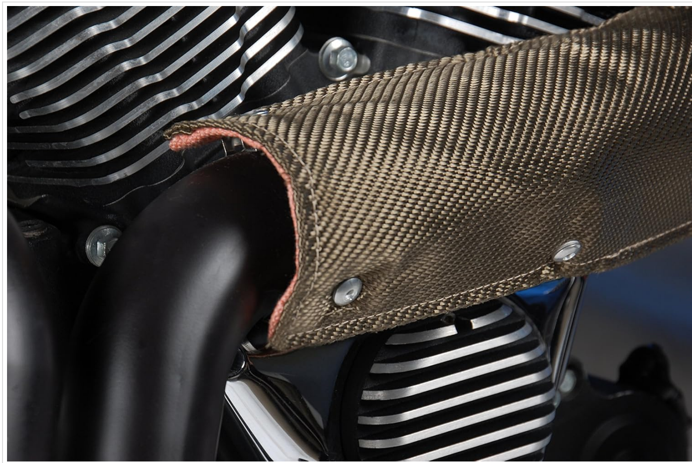
Image: The Titanium Pipe Shield applied to a motorcycle exhaust pipe, illustrating its application in tight engine bay spaces.
