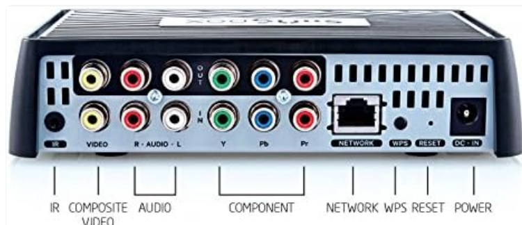
Figure 2: Rear view of the Slingbox M1, showing various input and output ports.
