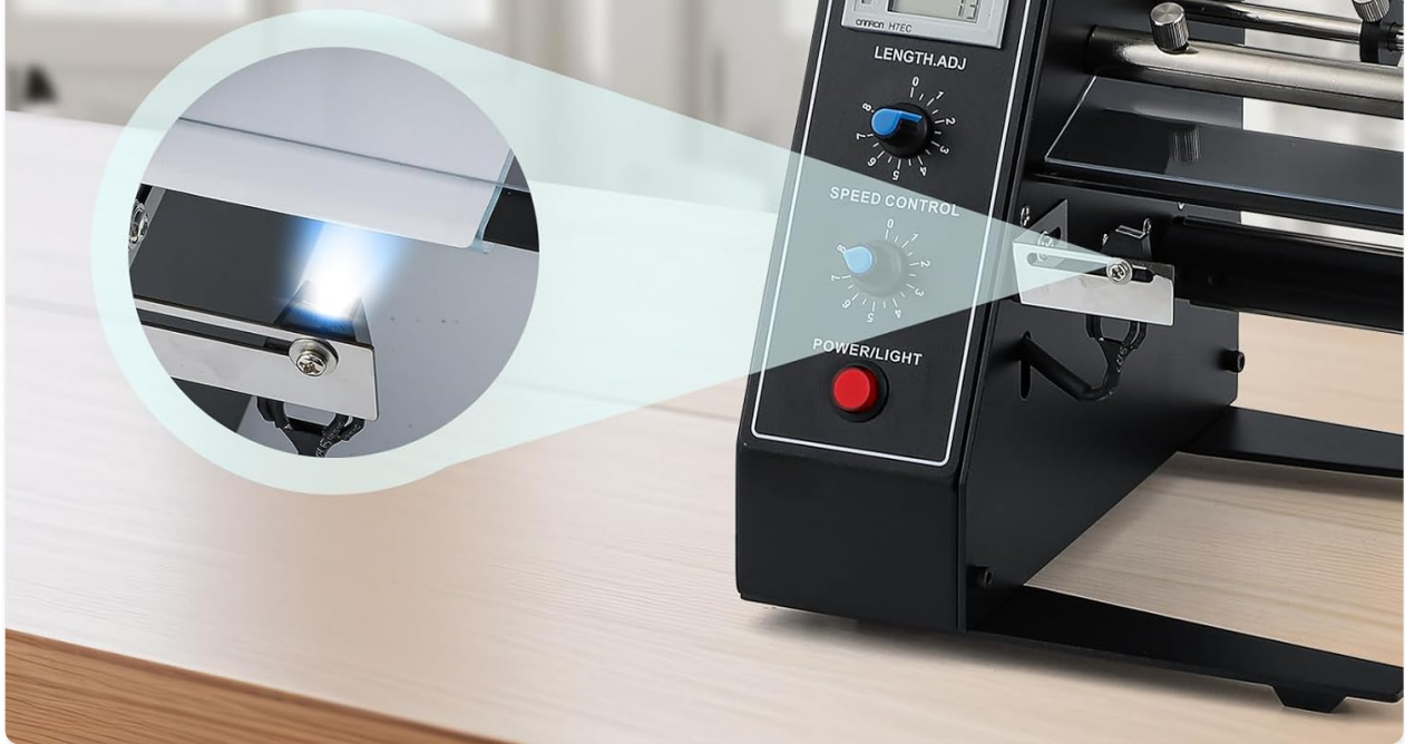
Figure 4: The auto-sensing feature ensures precise label peeling.
