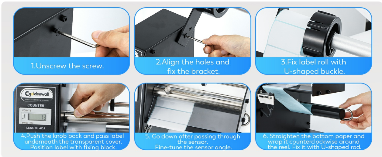
Figure 1: Step-by-step installation guide for the label dispenser components.
