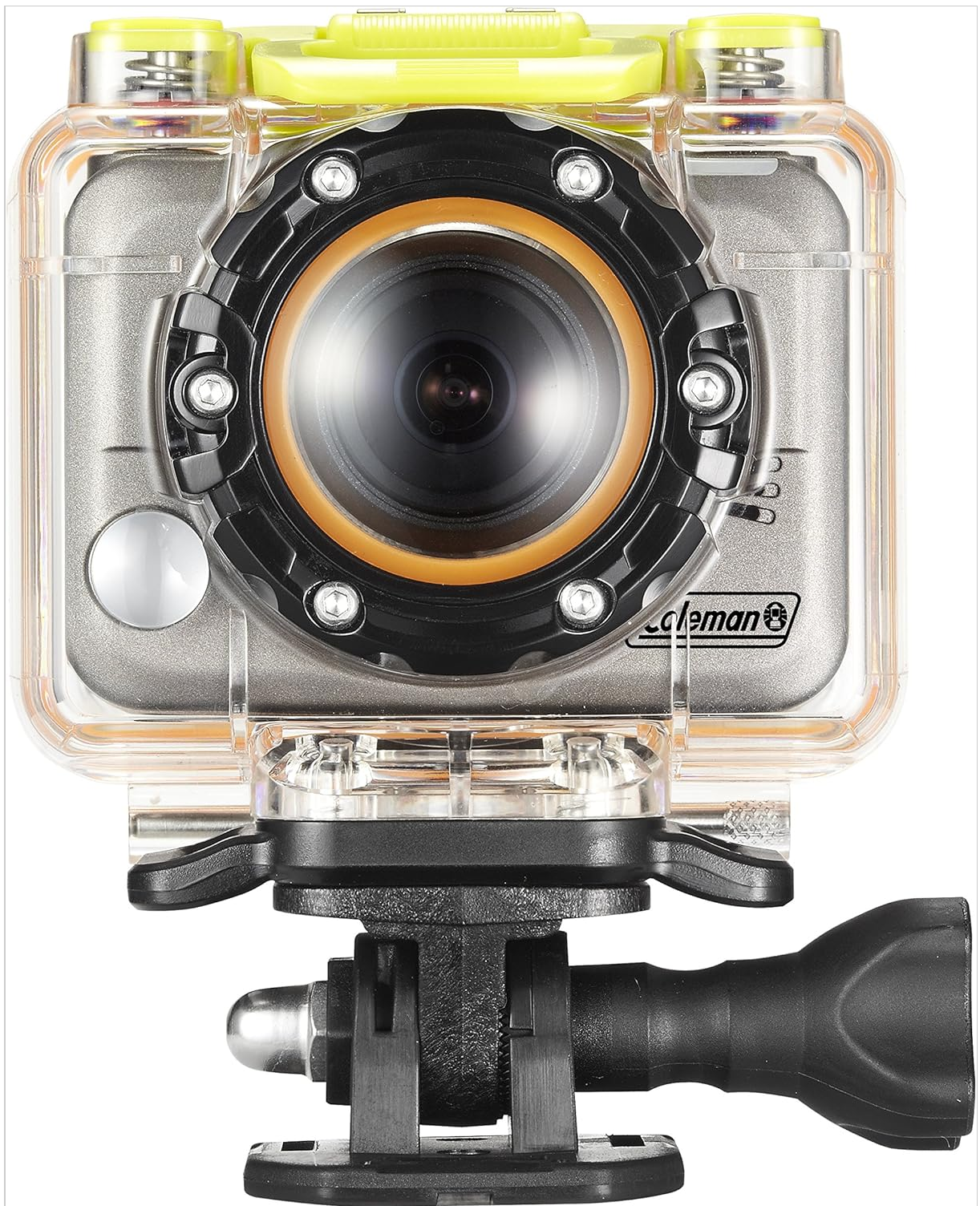
Figure 1: Front view of the Coleman Bravo CX10WP camera enclosed in its transparent waterproof housing. The lens is prominent in the center, surrounded by a black ring, with a yellow top latch visible.
