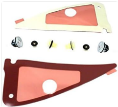
Image 3.3: A close-up of one of the black and white plastic mounting clips, designed to secure the spoiler to the vehicle body. It features a circular white head with a black base and a foam washer.
