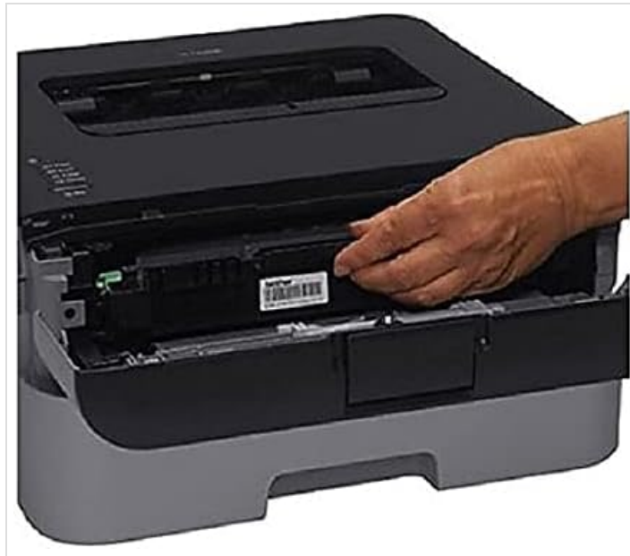
Figure 2.1: Proper insertion of the toner cartridge into the printer's designated slot.
