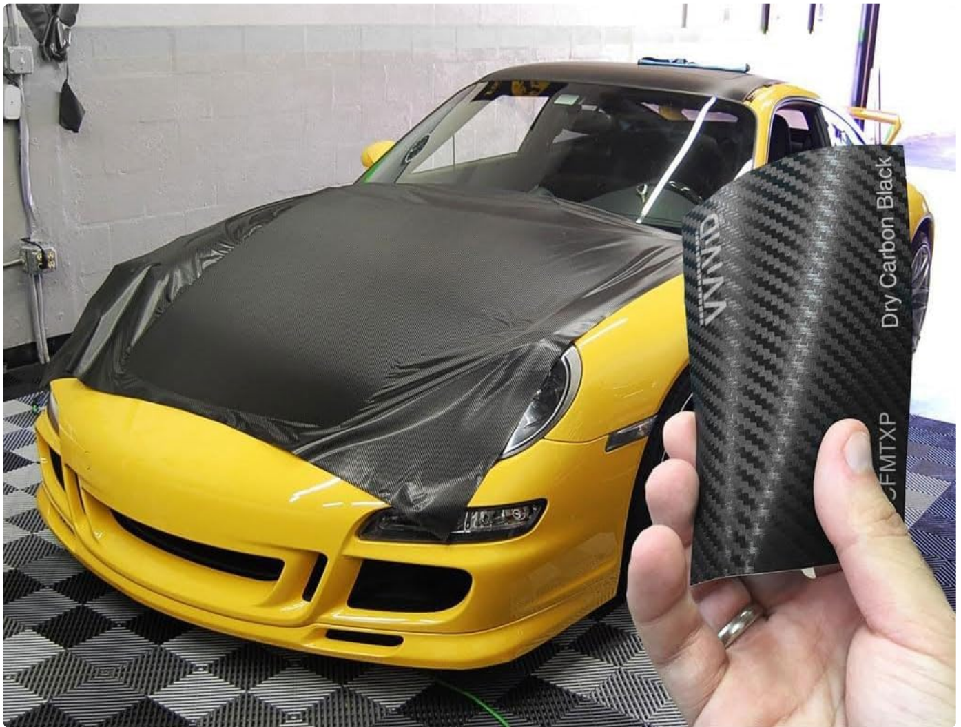
Image: Carbon fiber wrap being applied to a car hood, demonstrating the conformability of the material.
