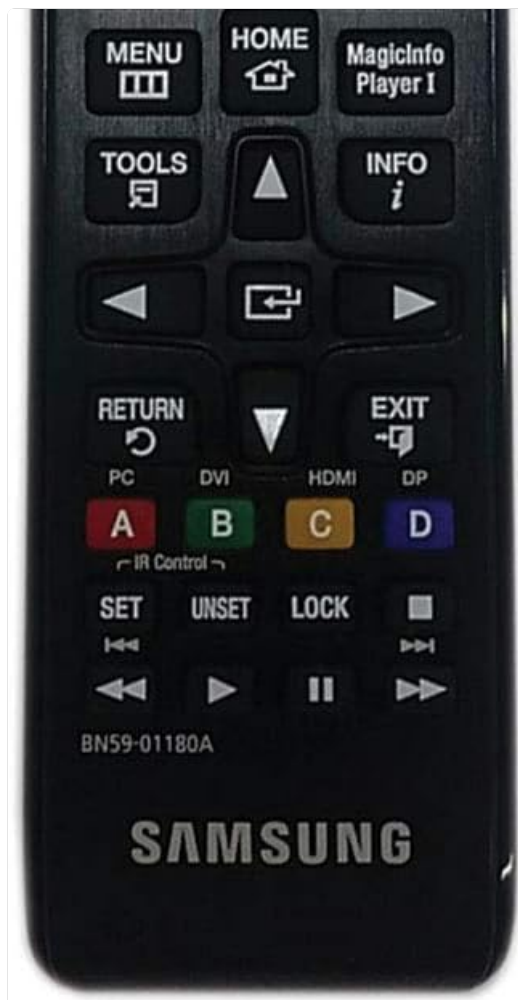
Figure 3: Close-up view of the lower section of the Samsung BN59-01180A remote control, showing navigation, return, exit, and color buttons.
