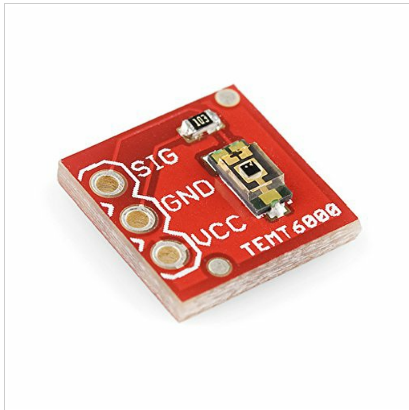
Figure 1: The SparkFun TEMA6000 Ambient Light Sensor Breakout Board. This image shows the small red PCB with three labeled pins (SIG, GND, VCC) on one side and the TEMA6000 sensor component and a resistor on the other side. The sensor is a small, clear component designed to detect light.
