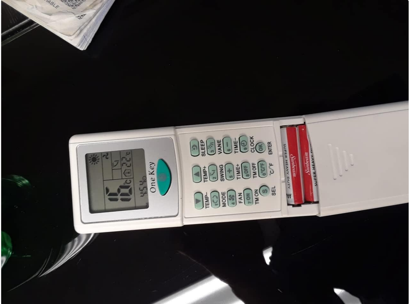
Figure 3: Battery compartment of the KT-E03 remote, showing where to insert AAA batteries.
