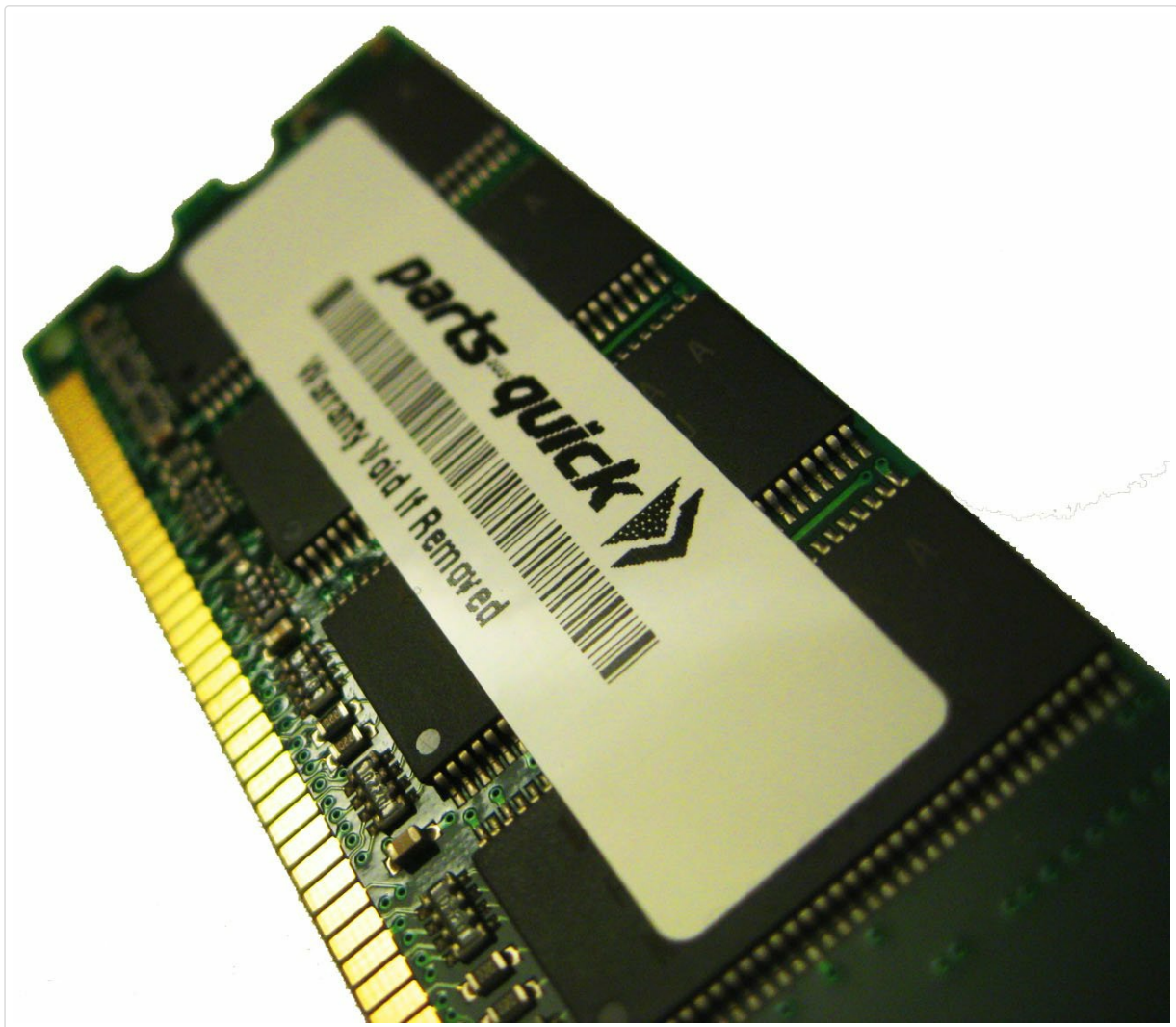
Image 1: The parts-quick 256MB DDR2 SO-DIMM memory module. This image displays the physical appearance of the memory stick, including its chips and connectors.
