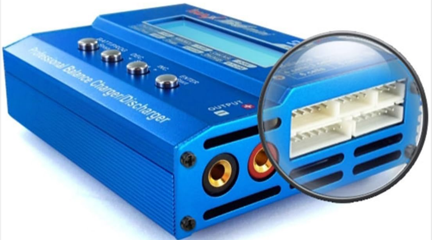
Image 4.2: Detailed view of the 2-6S XH plug-in balance sockets on the side of the charger, essential for balanced charging of lithium batteries.
