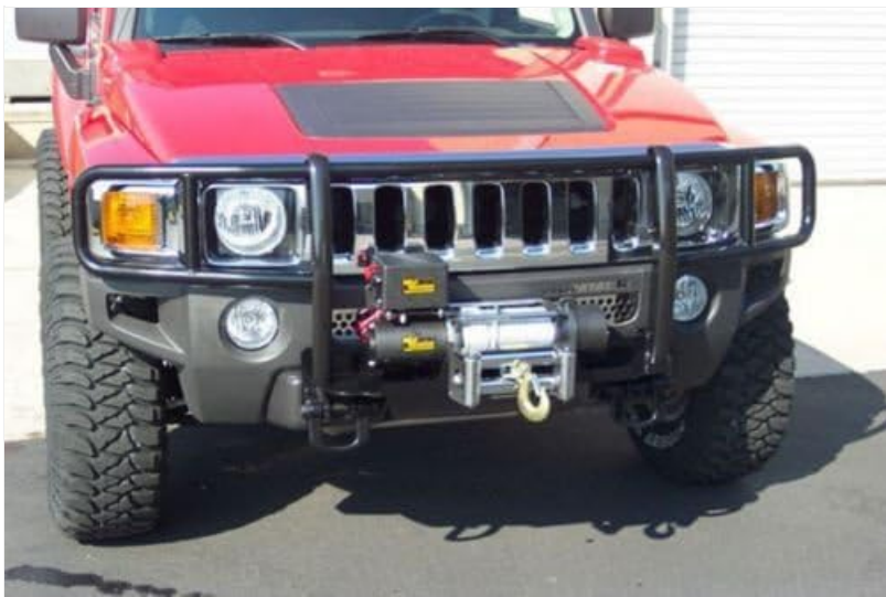
Image: A Hummer H3 featuring the TAC Grill Guard, with an additional winch mounted behind the guard, demonstrating compatibility with other accessories.
