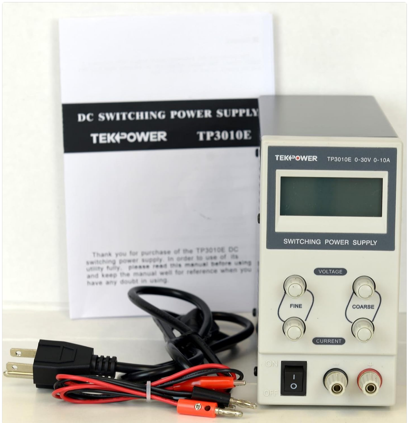
Figure 4.1: TP3010E Unit with Included Accessories.
