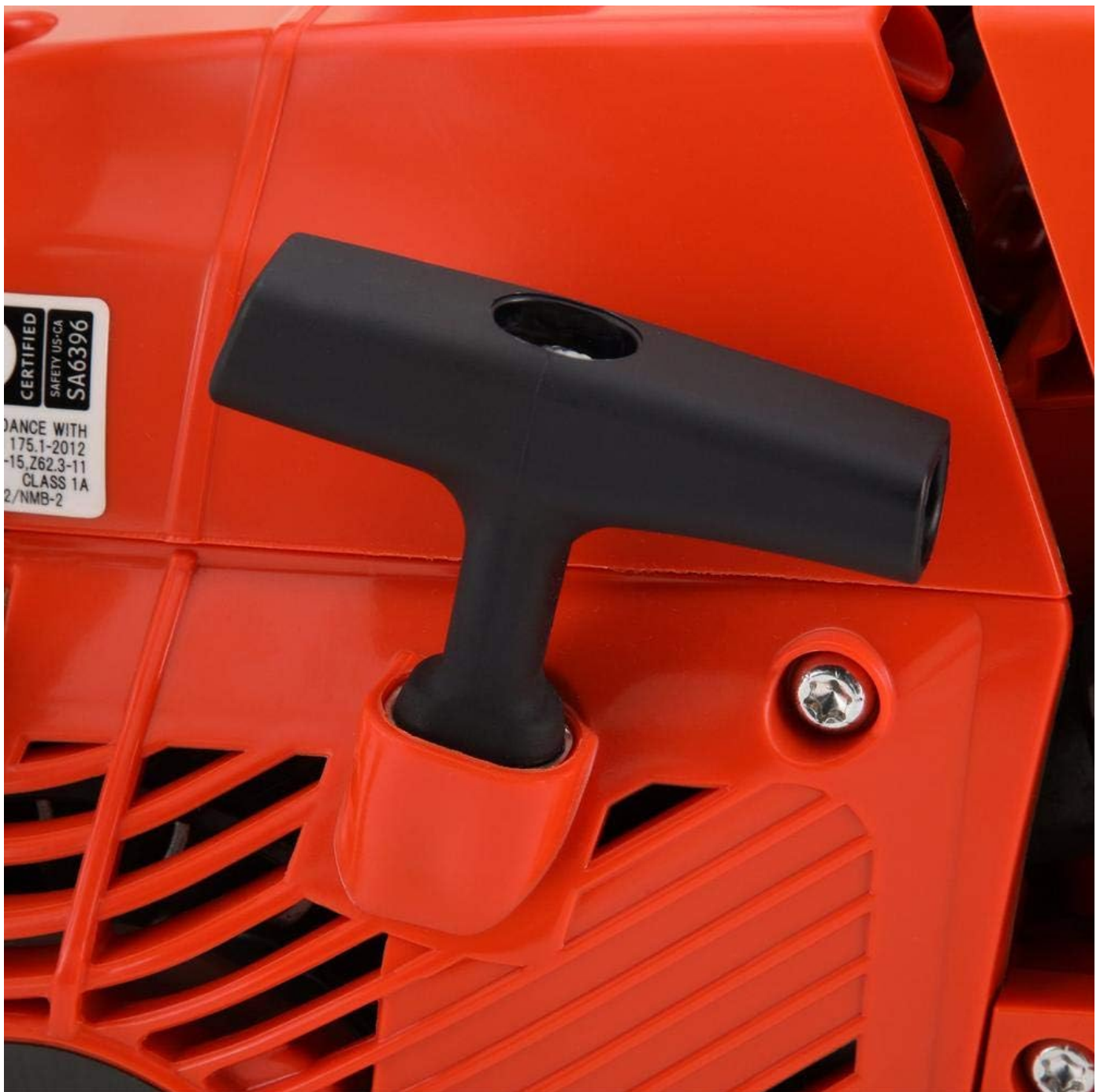
Image: Close-up view of the starter handle on the ECHO CS-590 chainsaw, used for manual engine ignition.
