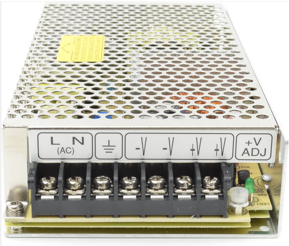
Image 3: Detailed view of the terminal block, showing AC input, DC output, and the voltage adjustment screw.
