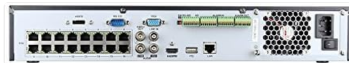
Figure 2.2: Rear panel of the NVR, illustrating the PoE ports for camera connections, HDMI and VGA outputs for display, USB ports, and the Ethernet port for network connectivity.
