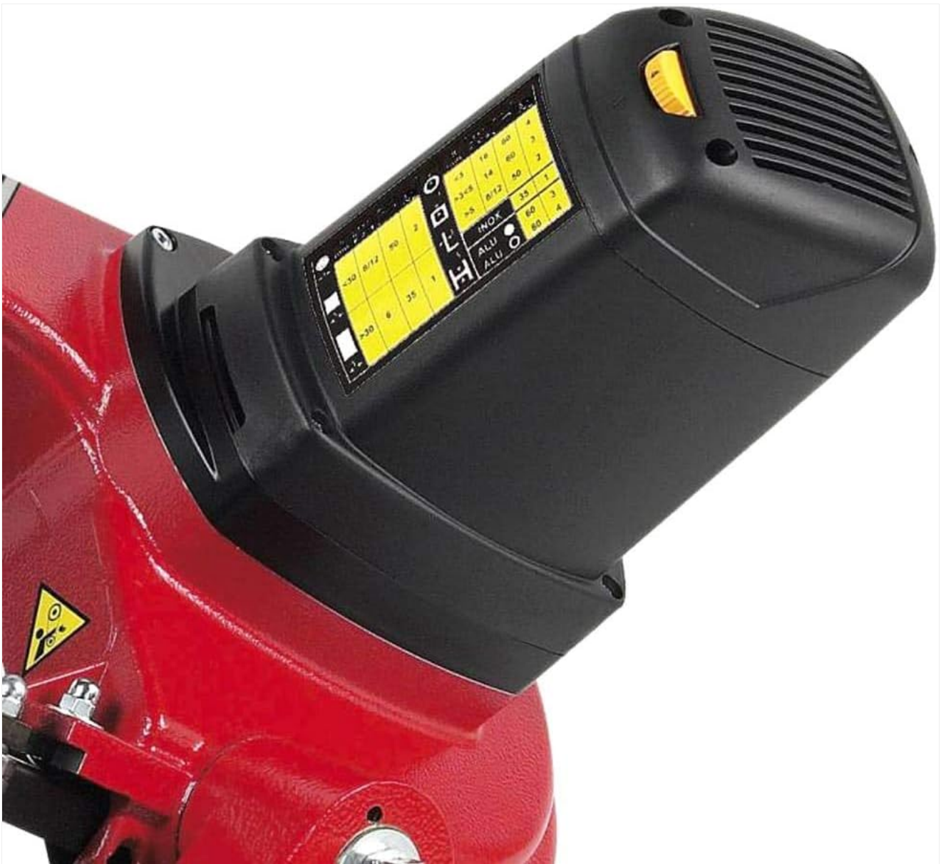
Figure 4: Close-up of the motor housing, showing the speed control and warning labels.
