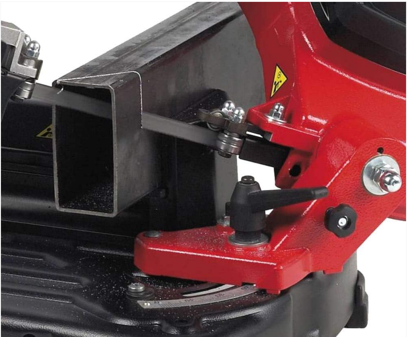
Figure 3: Detailed view of the blade and vice area, showing the blade path and clamping mechanism.
