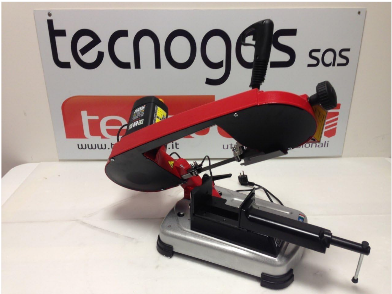
Figure 2: Side view of the FEMI 784XL, illustrating its compact design and the transport locking device.
