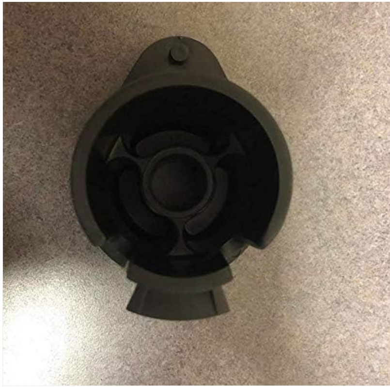
Figure 4.1: Top view of the Lincoln Electric KH720 Spindle Adaptor, showing the internal wire spool support structure.
