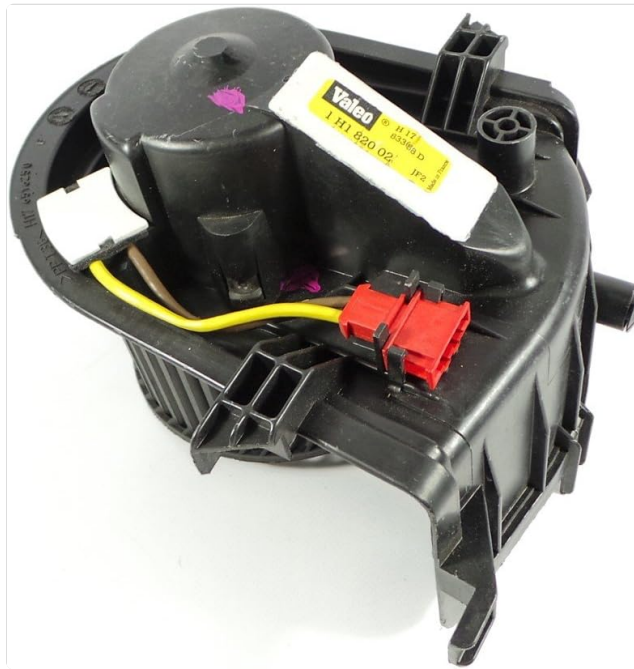
Figure 1: The Volkswagen Blower Motor 1H1-820-021, showing the main housing and electrical connectors. Note the yellow and brown wires leading to the red connector, and a white connector on the left.
