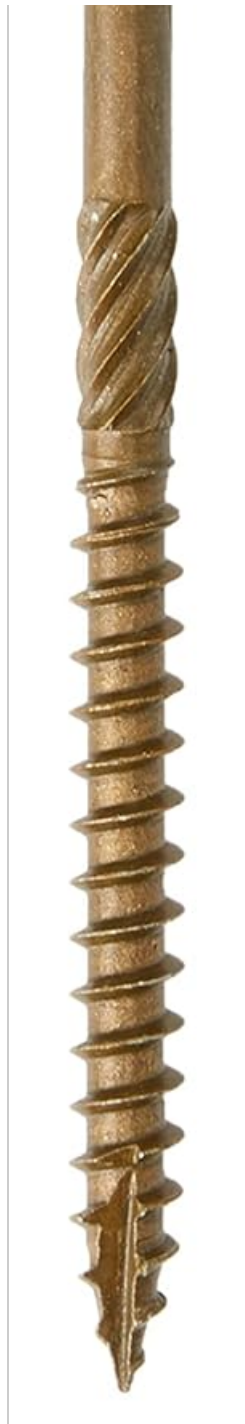
Figure 1: TIMCO Timber Screw 6.7 x 125. This image displays a single TIMCO timber screw, featuring a hex head with a fixed washer, a smooth shank, a helix shank section for debris removal, and a deep single thread leading to a sharp point. The screw has an exterior green organic coating.
