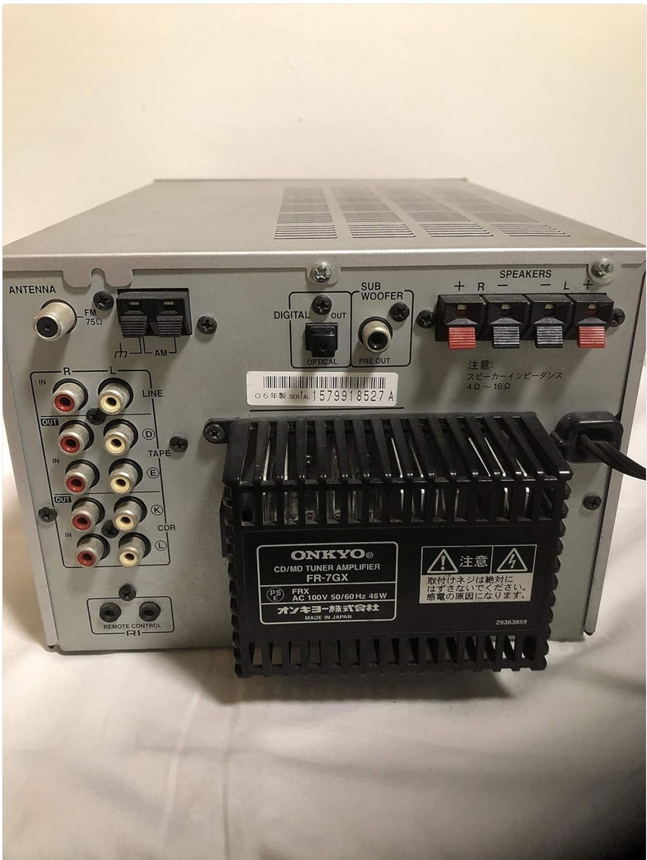
Figure 3.1: Rear view of the ONKYO FR-7GX, illustrating the various connection terminals including speaker outputs, analog inputs/outputs, digital output, and antenna connections. Proper connection of these terminals is essential for the unit's functionality.
