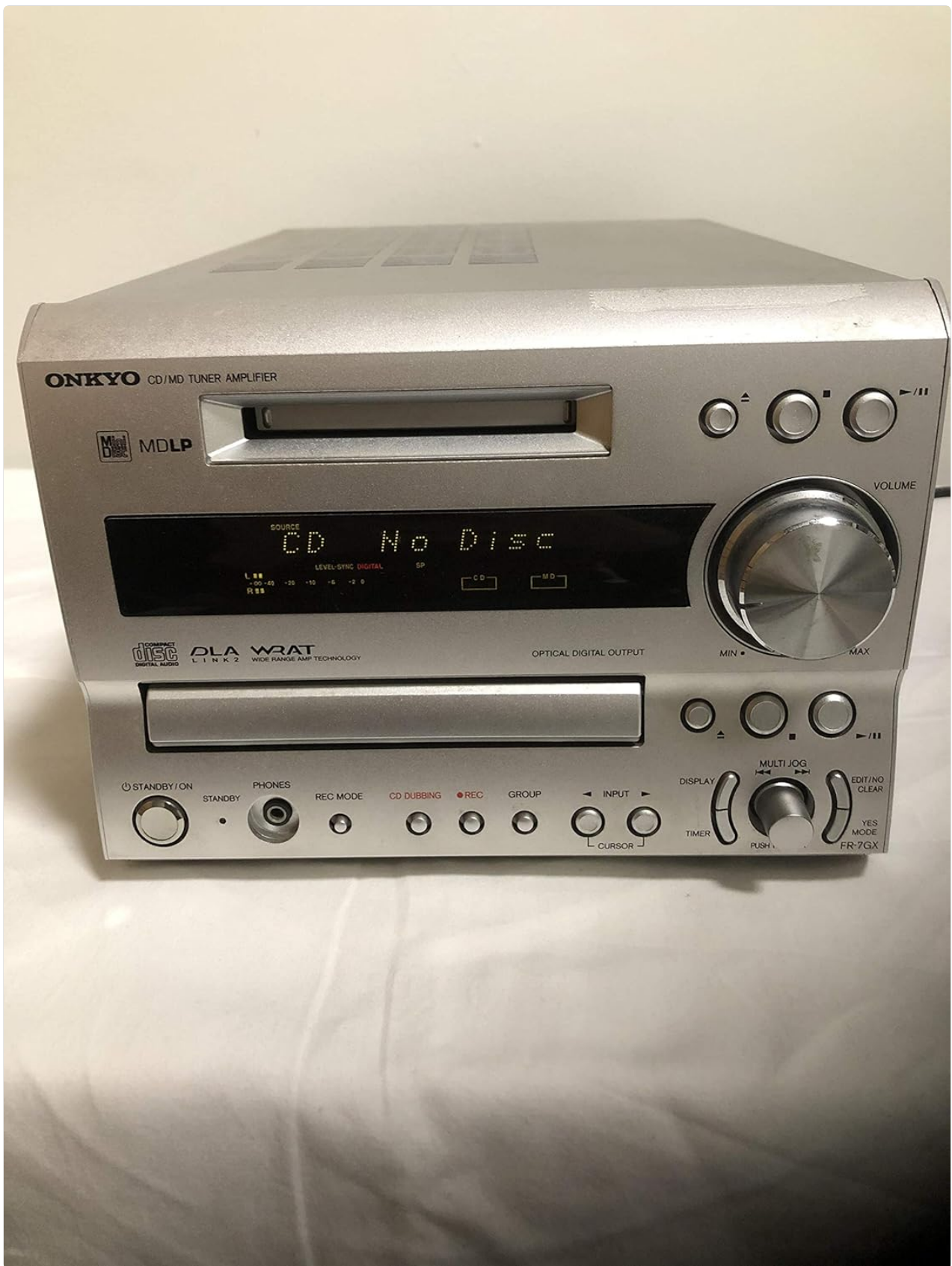
Figure 1.1: Front view of the ONKYO FR-7GX CD/MD Tuner Amplifier. This image shows the main unit with its silver finish, the CD tray, MD slot, display panel, and various control knobs and buttons, including the large volume dial on the right.
