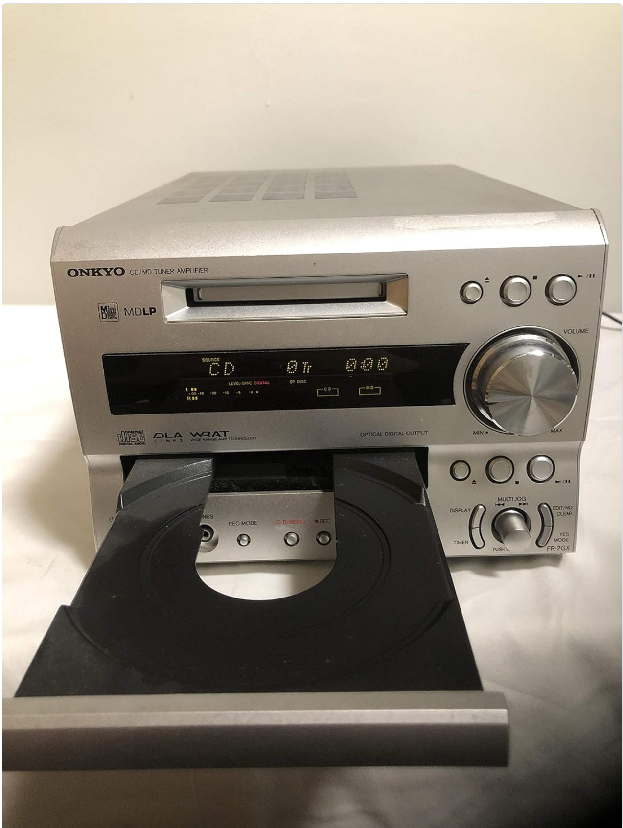
Figure 4.1: Front view of the ONKYO FR-7GX with the CD tray extended. This illustrates the mechanism for loading compact discs for playback.
