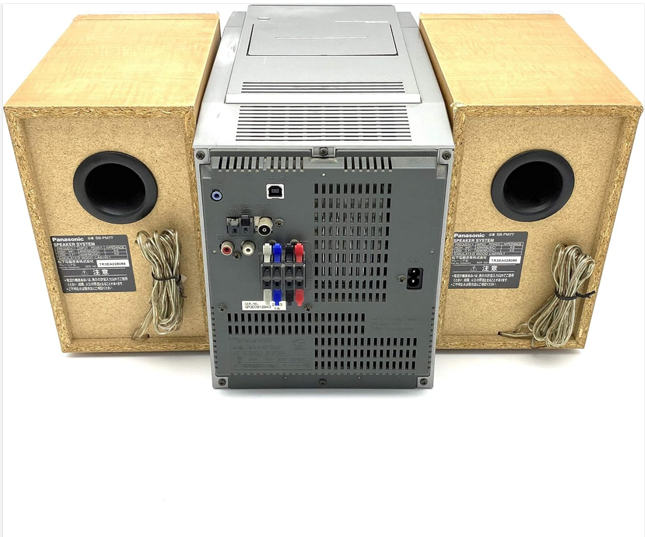
Image: Rear panel of the main unit showing the speaker terminals and other input/output ports. The speaker cables are connected to the color-coded terminals.
