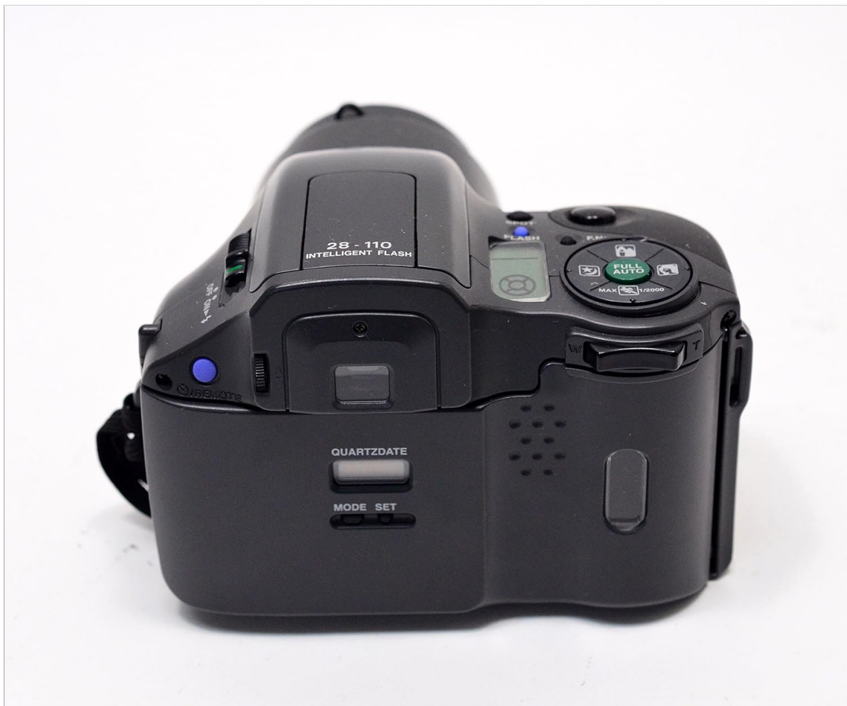
Image: Rear-top view of the Olympus IS 10 camera, highlighting the control panel with buttons for flash, full auto mode, zoom, and the Quartzdate settings. The LCD display is also visible.
