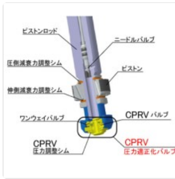
Image 2.2: Diagram illustrating the damping force characteristics and CPRV function.
