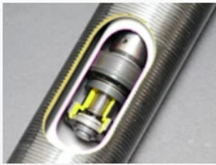
Figure 2: Key features of the CUSCO Street ZERO A coilover, including damping adjustment and CPRV.
