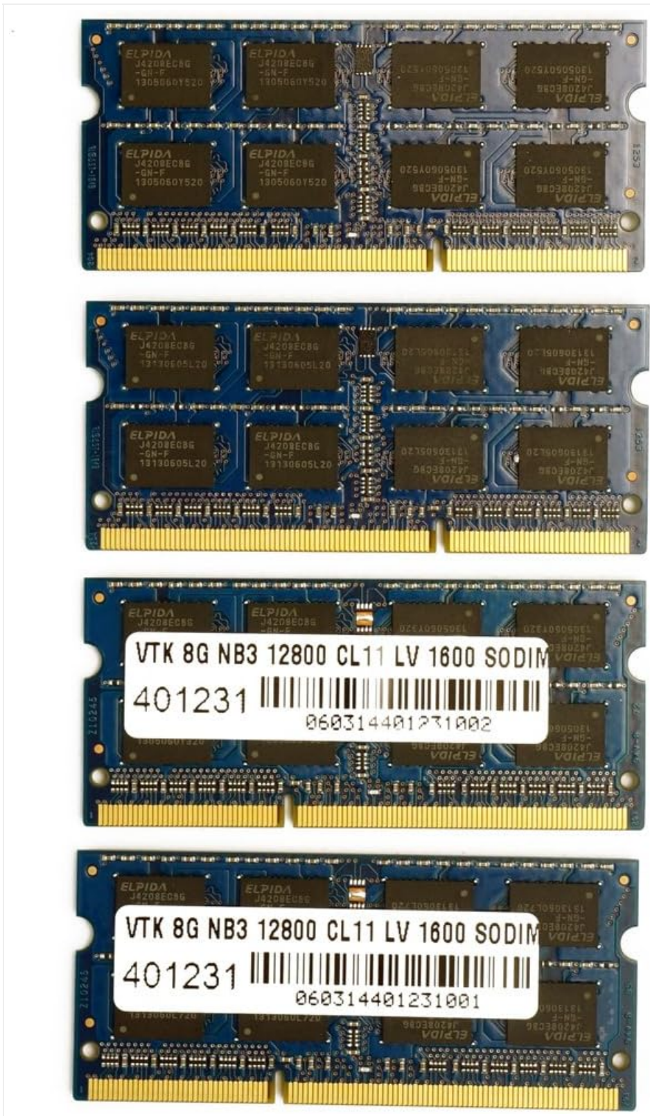
Figure 1: Four VisionTek 8GB DDR3 SODIMM memory modules. Each module features multiple black memory chips on a blue circuit board, with a white label indicating "VTK 8G NB3 12800 CL11 LV 1600 SODIM" and a unique serial number.
