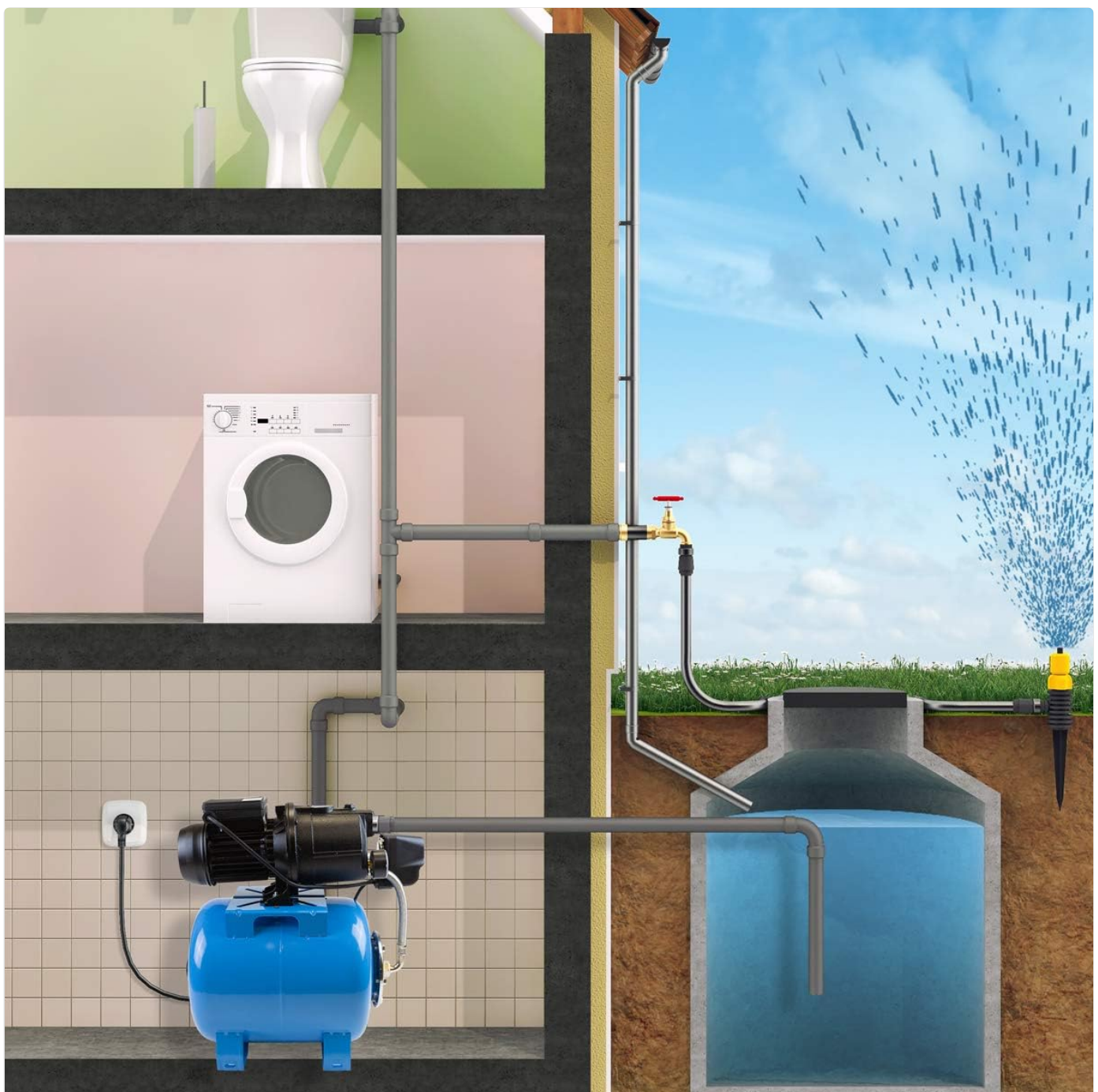
Figure 5.2: Example application diagram illustrating the Waterpress 750's integration into a domestic water supply and irrigation system.
