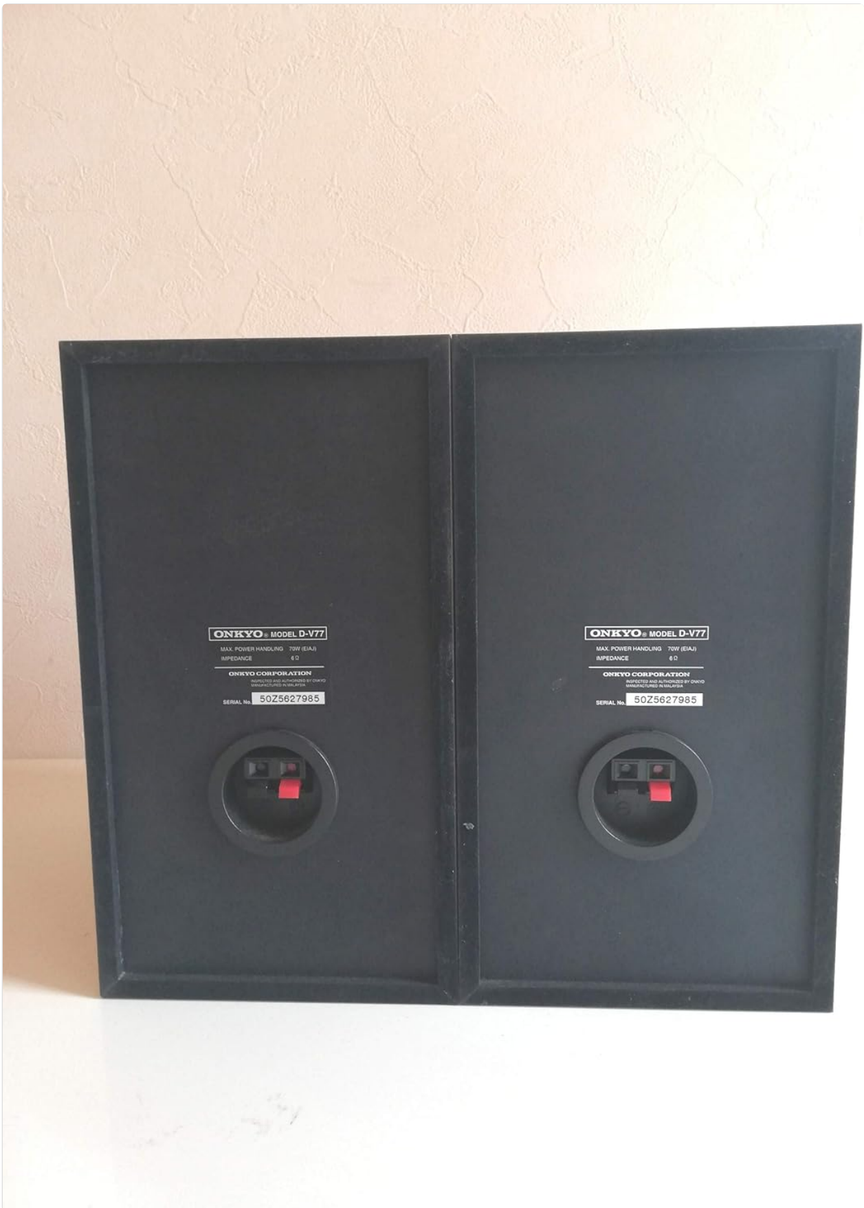
Figure 4.2: Rear view of the D-V77 speakers, showing the spring-clip speaker terminals for connection.
