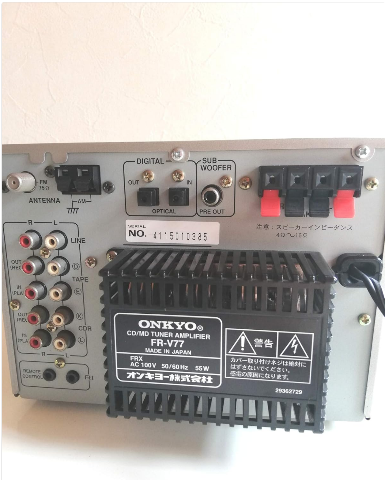
Figure 2.1: Rear panel of the FR-V77 main unit, highlighting the speaker terminals and the electrical safety warning.
